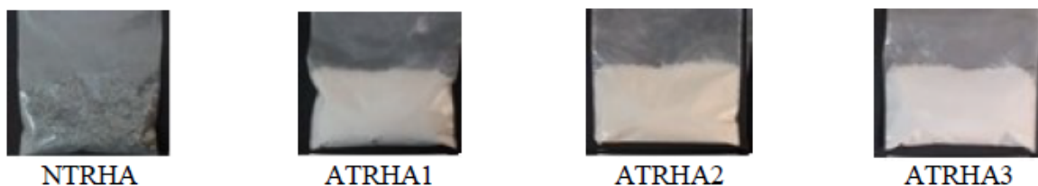
Color difference between NTRHA and ATRHA 1, 2 and 3 samples that combusted at 800°C for 2 hours.
