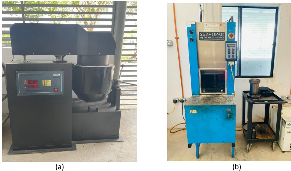
Fig. 1. Figure mixing and compaction sample (a) 20L heavy-duty mixer (b) Superpave gyratory compactor
