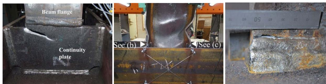
**Fig. 4.** Damage Model of H-profile of Beam-to-column Connection[25]
