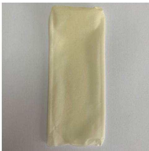
**Fig. 4.** Coherent, smooth and uniform surface of vulcanized PMMA graft NR film
