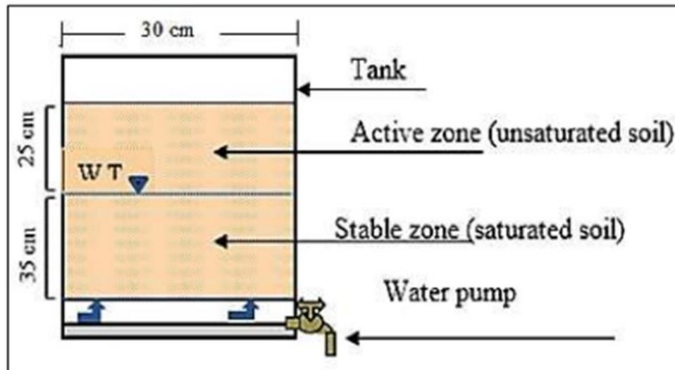
Fig. 1. Physical model for laboratory testing
