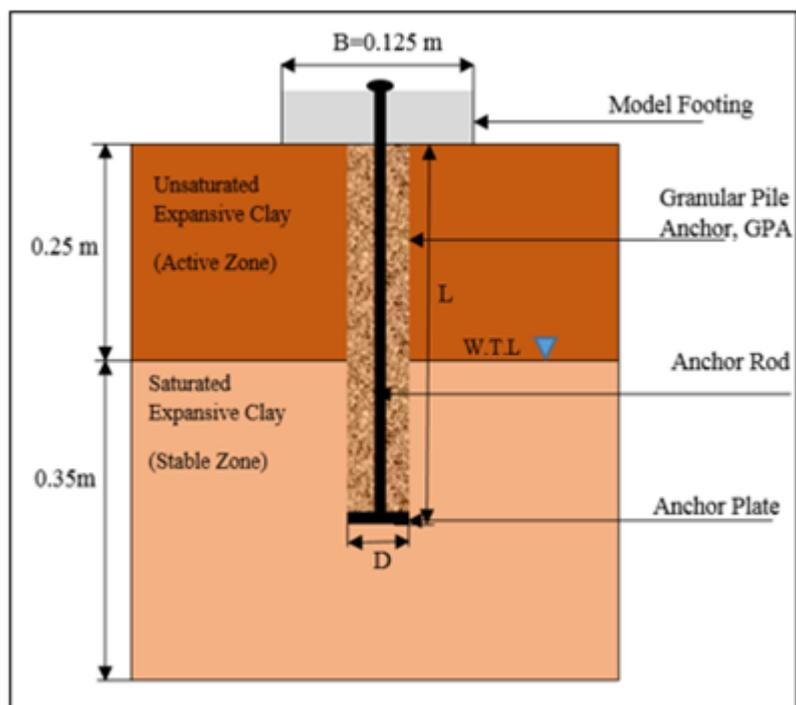
Fig. 3. The model details of the numerical modelling test
