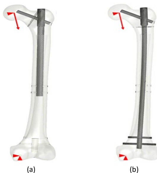
Fig. 6. Nail with distal fixation screw (a) short, 13mm diameter (b) long, 10mm diameter
