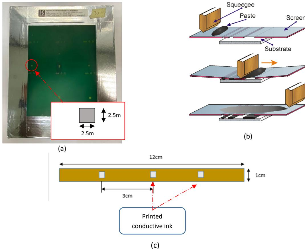
**Fig. 3.** Printing procedure of conductive ink onto copper substrate using silkscreen and squeegee (a) silkscreen with printed images to print conductive ink onto copper substrate (b) Printing technique using silkscreen and squeegee to print conductive ink on copper substrate (c) Printed conductive ink on 12cm x 1cm copper substrate with 3cm distance apart from each other
