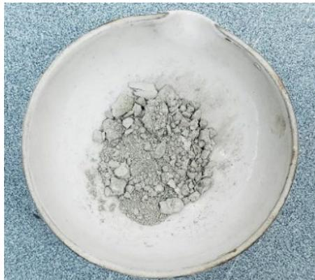
**Fig. 2.** powdered texture achieves after being treated in UF55 universal oven for 1 hour at 250  $^{\circ}\text{C}$
