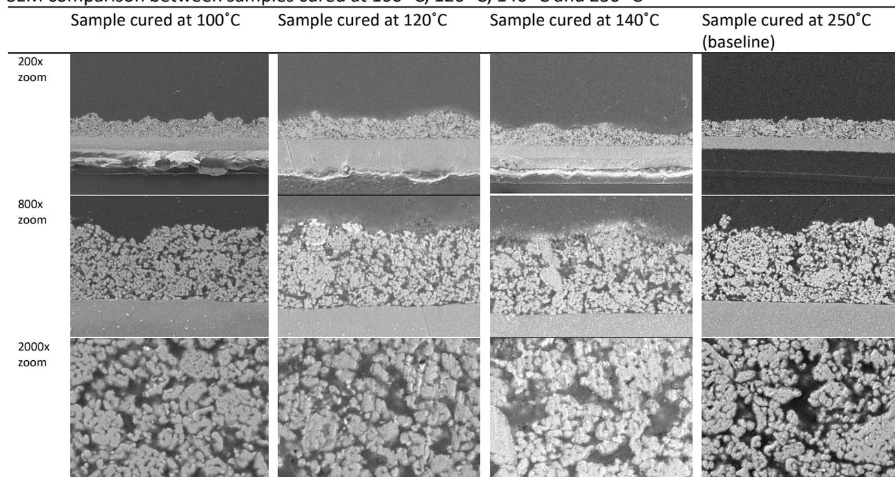
At 2000x magnification, the particles of the sample cured at 100 °C showed a better bond between each other, as suggested by Table 3 below. This result shows a well-interconnected structure that produces effective conductivity. However, it is worth noting that the surface of the printed ink appears to be rough at 200x magnification, which may contribute to how the GNPs disperse [13,14].
