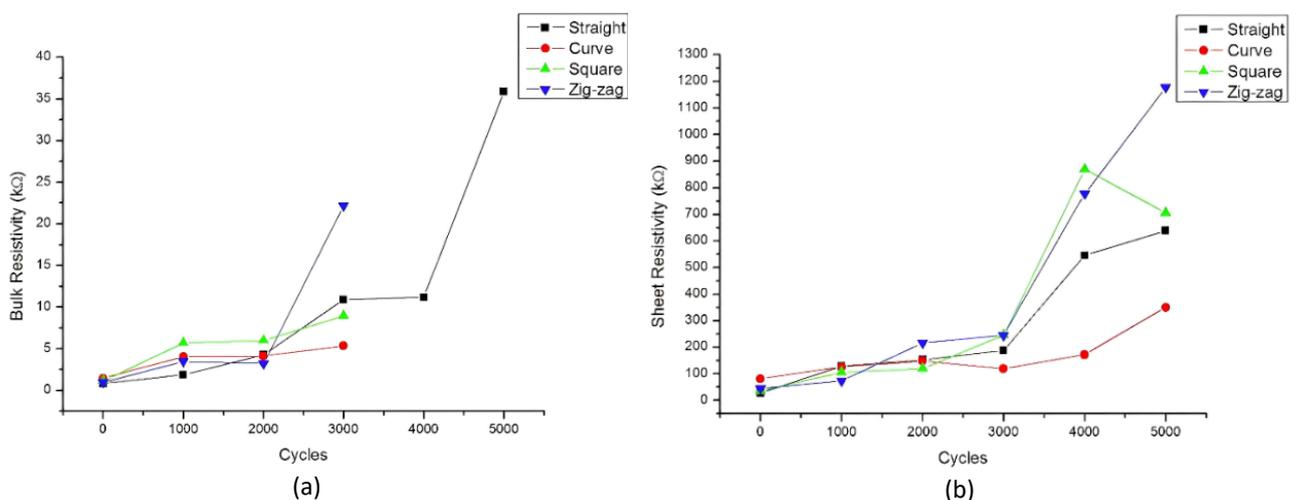
Fig. 1. Resistivity over cyclic bending (a) bulk resistivity (b) sheet resistivity
