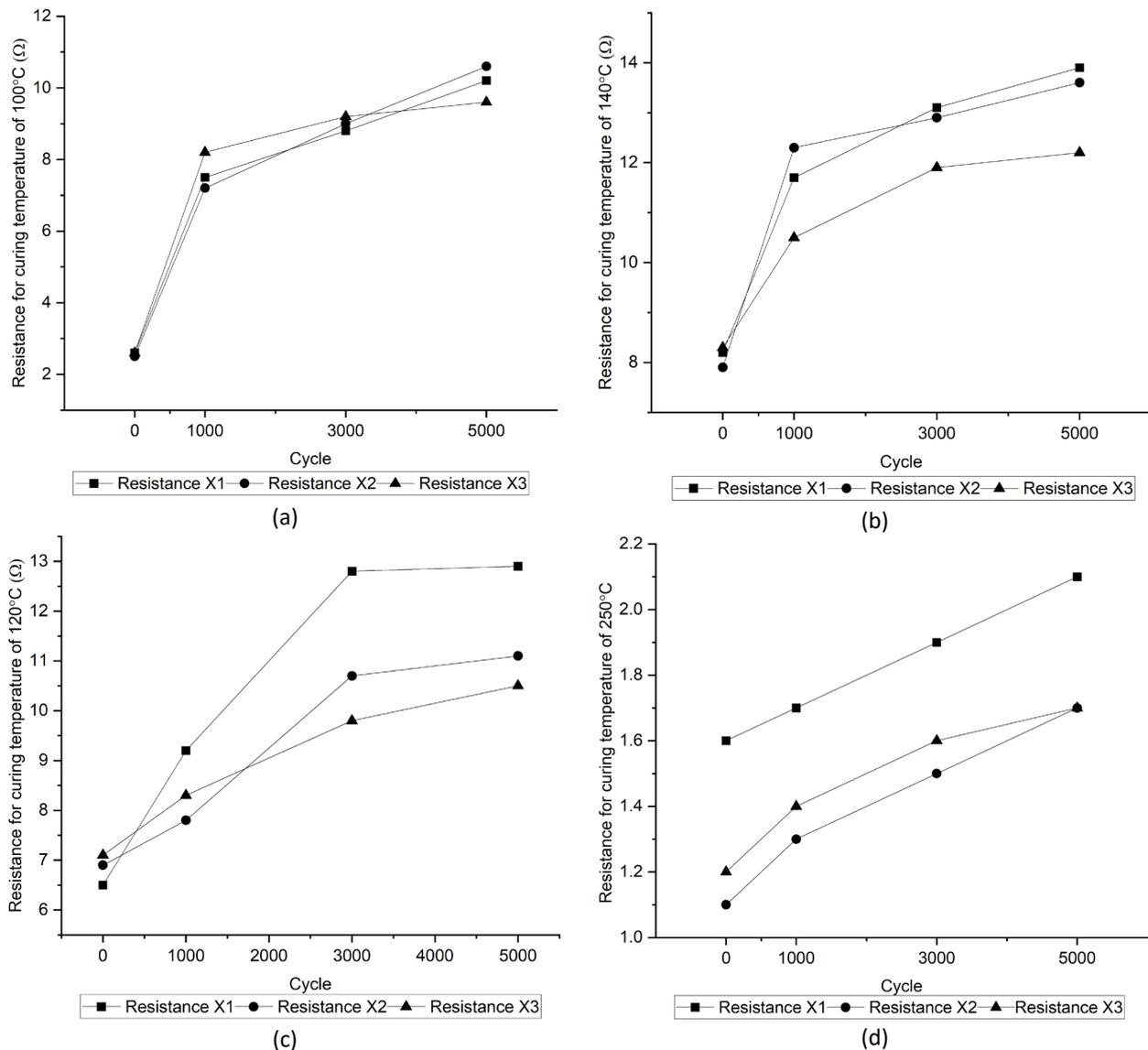
**Fig. 6.** Resistance over cyclic bending test (a) sample cured at 100 °C (b) sample cured at 120 °C (c) sample cured at 140 °C (d) sample cured at 250 °C
