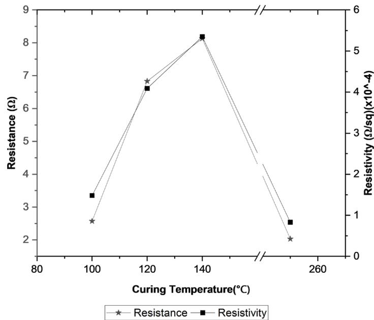
**Fig. 5.** The resistivity increases gradually as the curing temperature increases, except for the sample cured at 250 °C, where sintering occurs, resulting in a significantly lower resistivity
