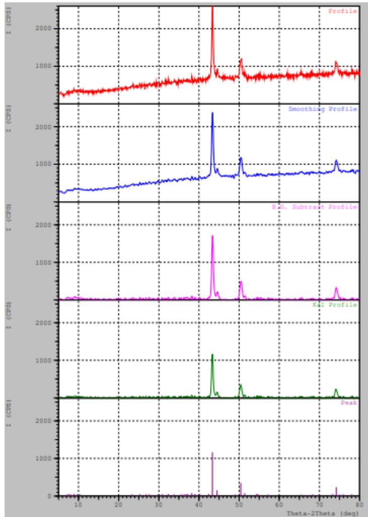
Fig. 6. X-ray Diffraction pattern for the Weldment
