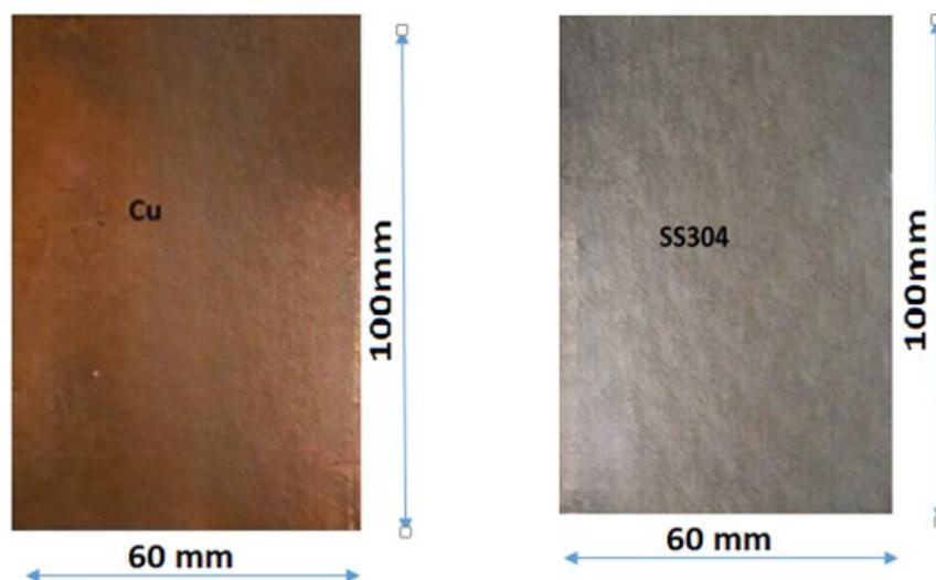
Fig. 1. Specimen for welding
