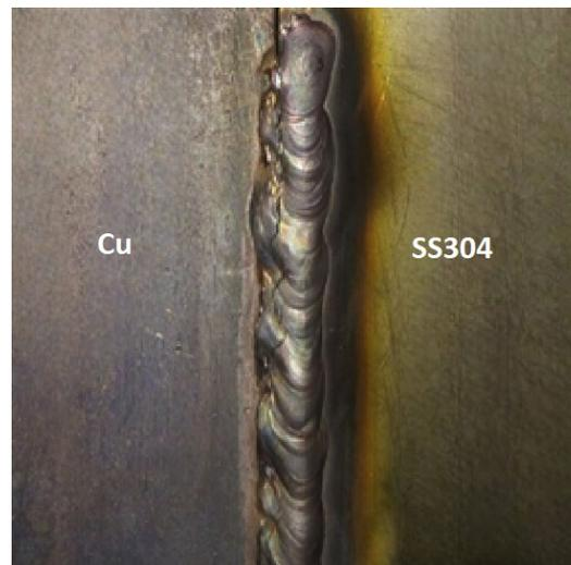
**Fig. 4.** Copper and SS304 Joint with filler
