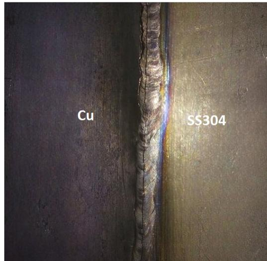
**Fig. 3.** Copper and SS304 Joint without filler
