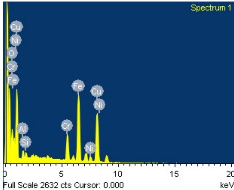
Fig. 7. EDX spectrum showing elements in the intermetallic compound of GTAW specimen
