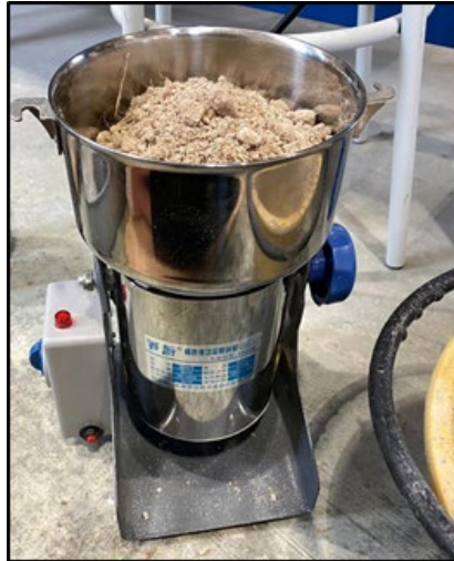
Fig. 1. Raw sago waste ground using grinder machine
