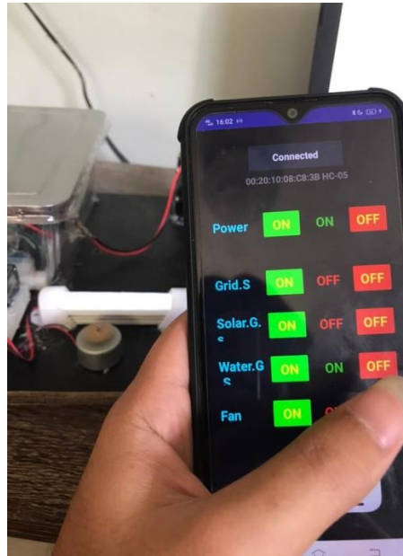
Fig. 11. Lamp and the motor are turned on when switching to the water generation supply
