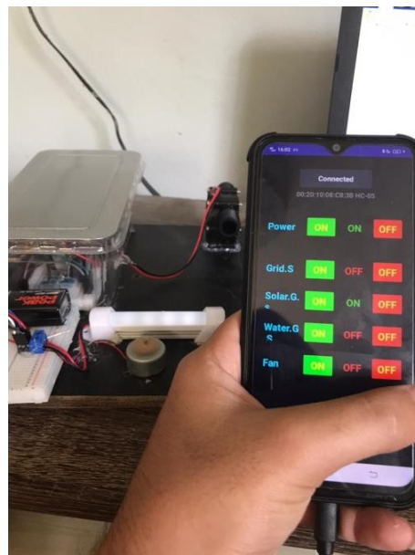
Fig. 10. Lamp and the motor are turned on when switching to the solar generation supply
