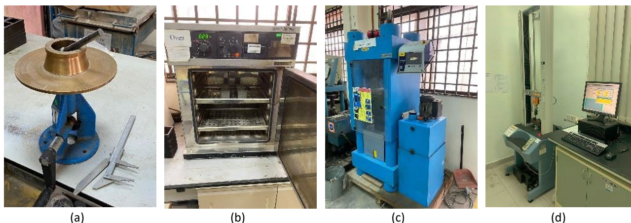
Fig. 2. (a) Flowability Test (b) Hardened Density Test (c) Compressive Strength Test and (d) Flexural Strength Test
