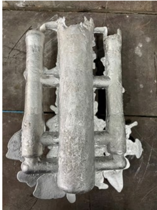
Fig. 4. As-cast after Cooling-slope experiment
