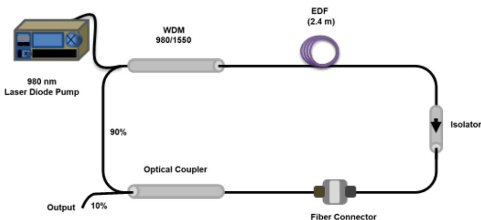
**Fig. 2.** Ring Laser Cavity Configuration
