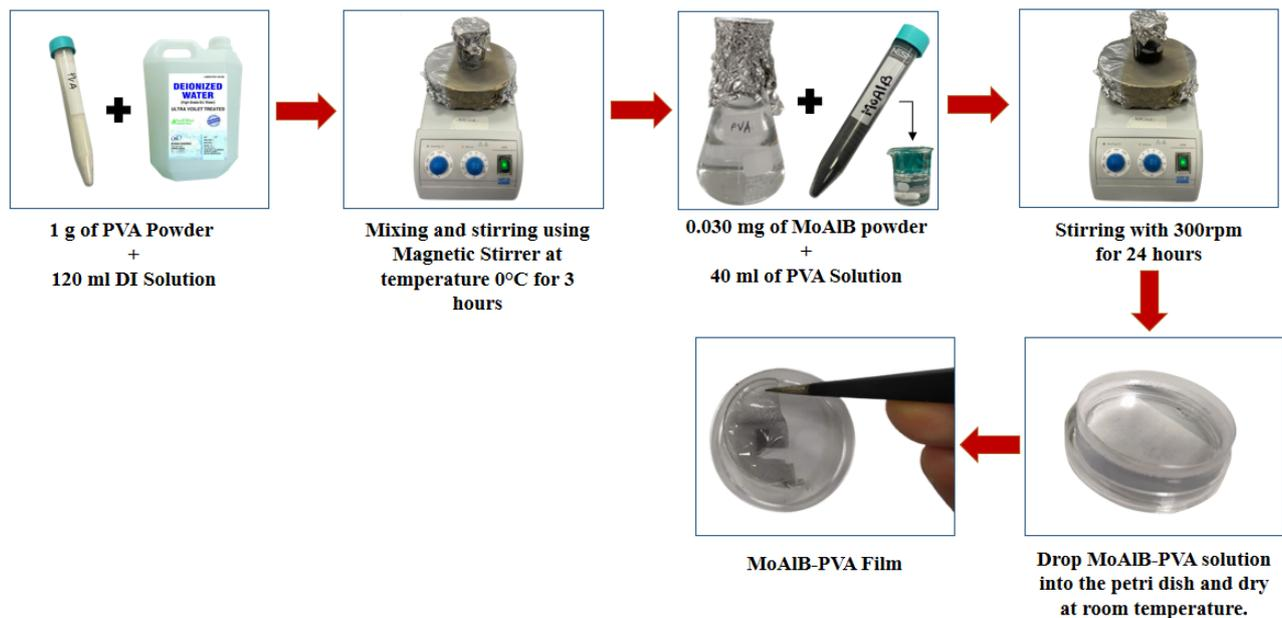
**Fig. 1.** Fabrication process to develop MoAlB thin film
