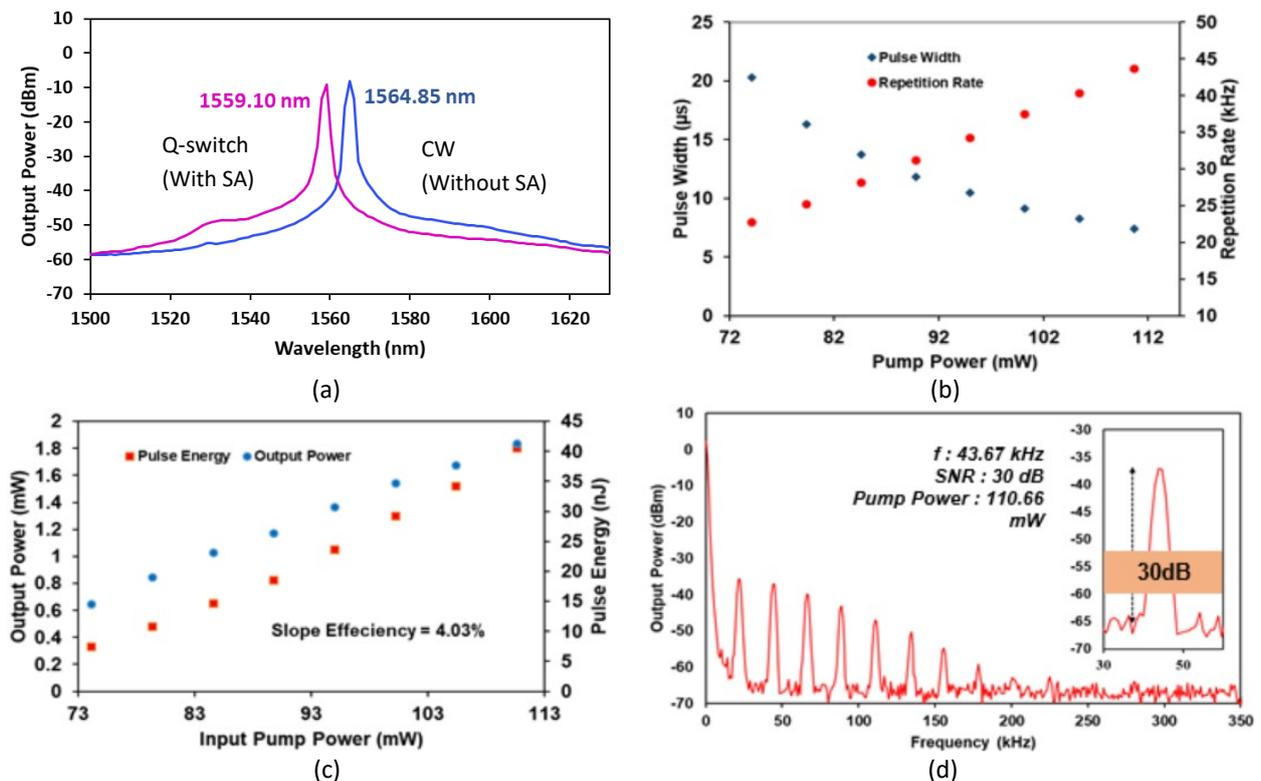
**Fig. 3.** Performances of Q-switched EDFL (a) Output Spectrum (b) Repetition rate and pulse width (c) Output power and pulse energy (d) RF Spectrum
