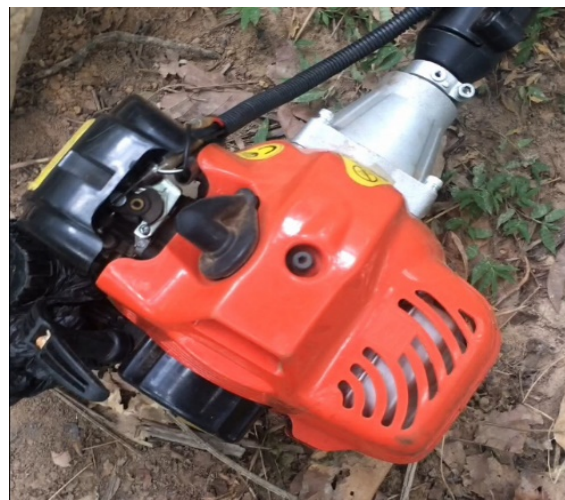
Fig. 5. Picture of the 1.3 Hp gasoline engine (2-stroke) of the mechanical harvester
