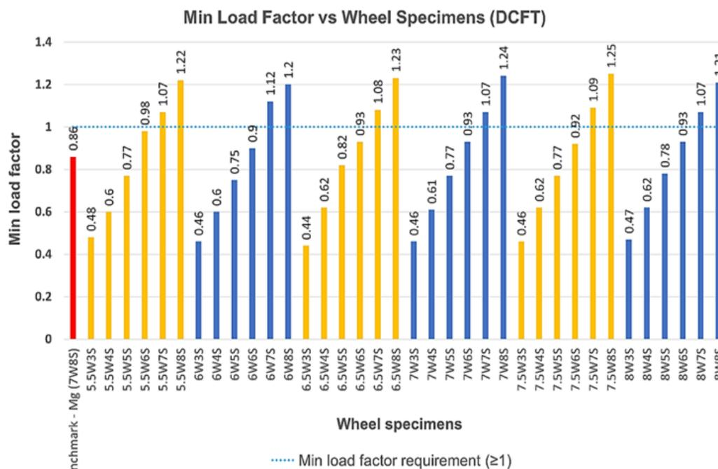
Fig. 8. Plot of minimum load factors against wheel specimens
