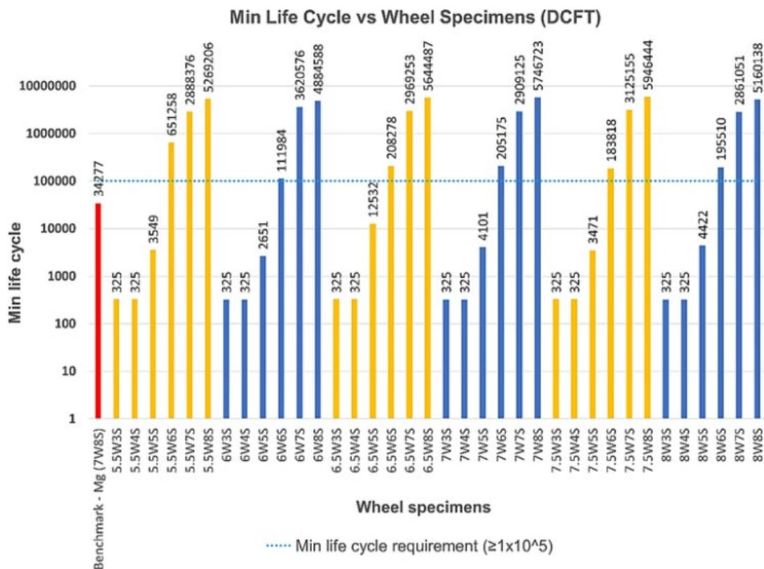
Fig. 7. Plot of minimum life cycles against wheel specimens
