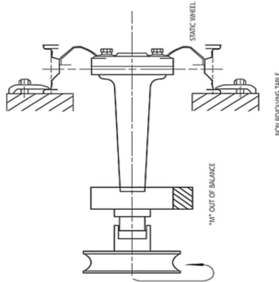
**Fig. 1.** Contour Setup of Dynamic Cornering Fatigue Testing Machine (Cai, Wang, Huang, Liu, & Liu)
