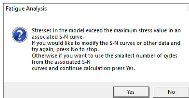
Fig. 6. Fatigue analysis problem during the 3S and 4S wheels' simulations
