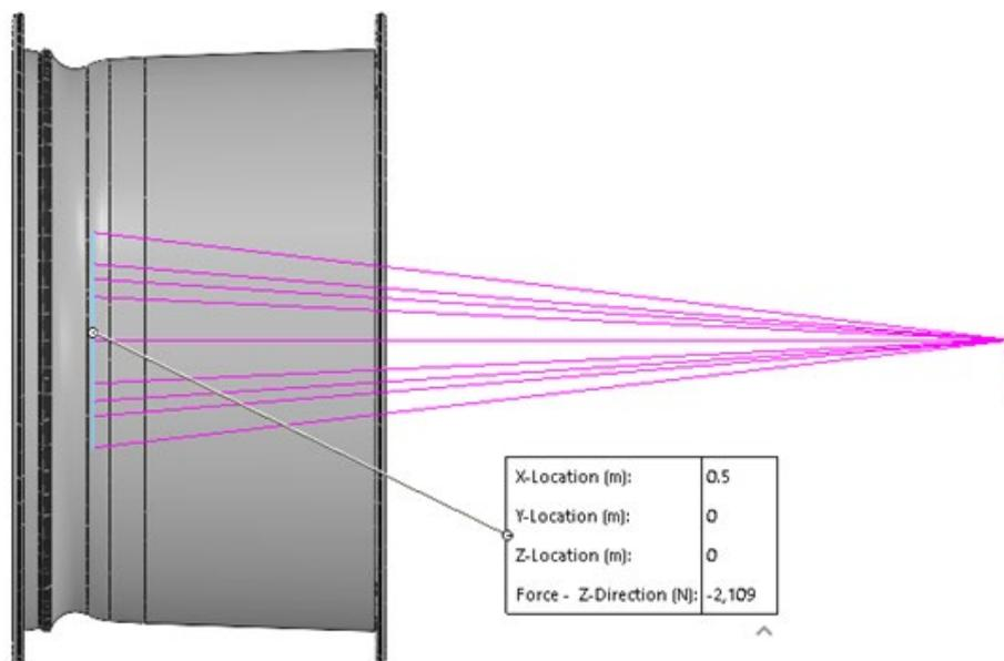
**Fig. 2.** The bending moment was created by using the "Remote Load" function in SolidWorks (Bagherzadeh, Murugesan, & Deka)
