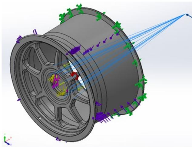
**Fig. 4.** The isometric view of the test setup for the DCFT
