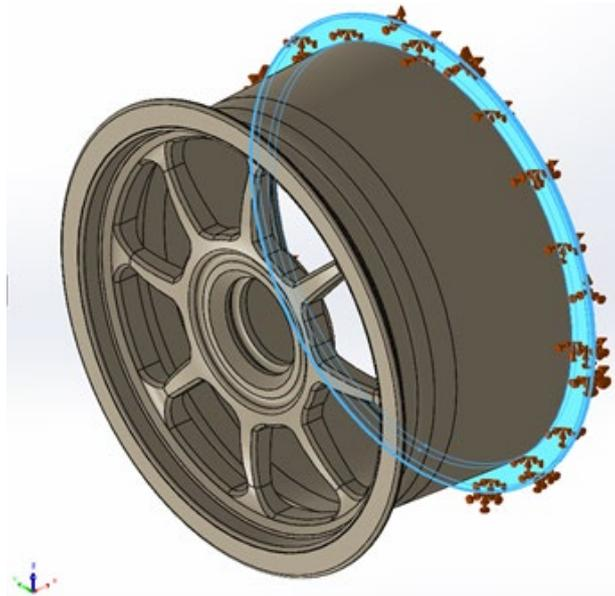
**Fig. 3.** The lower wheel flange was constrained during the analysis
