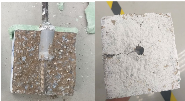
Fig. 3. The failure mode of splitting tensile specimens
