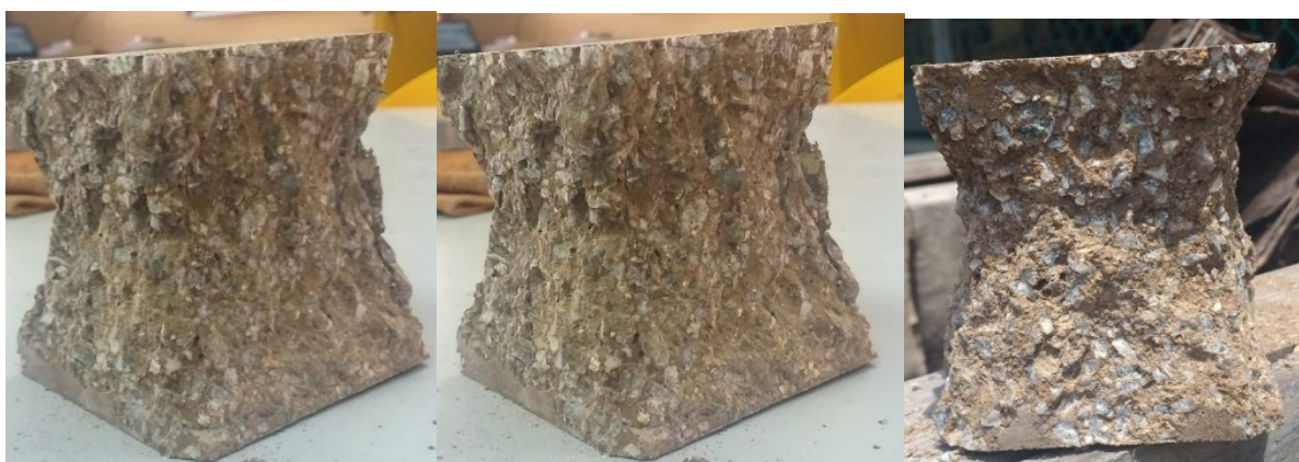
Fig. 1. Cube specimens failure mode
