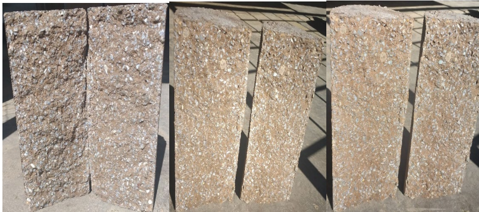
Fig. 2. The failure mode of splitting tensile specimens
