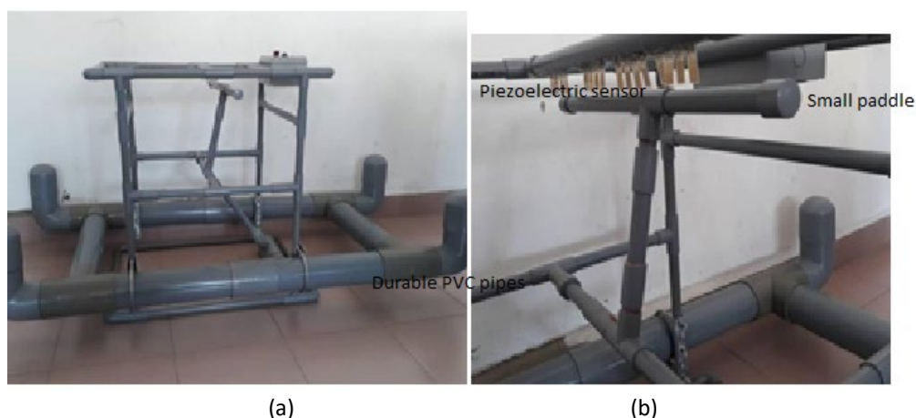
Fig. 3. (a) PEH-2 integrated with a floating device and (b) small paddle initiating energy harvesting from the piezoelectric sensor film
