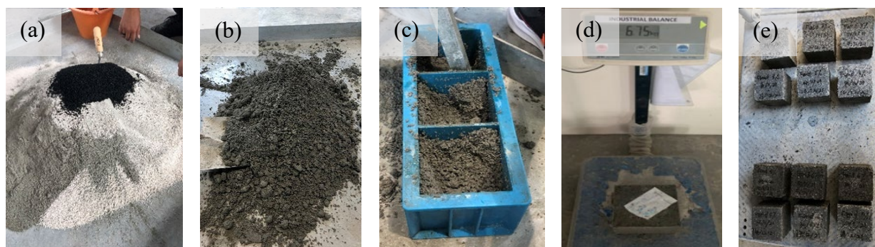
Fig. 6. Process of (a)mixing raw materials, (b)mixing with water ratio, (c)compacting each layer using a tamping rod, (d)weighing cube sample, and (e)ready place in the curing tank
