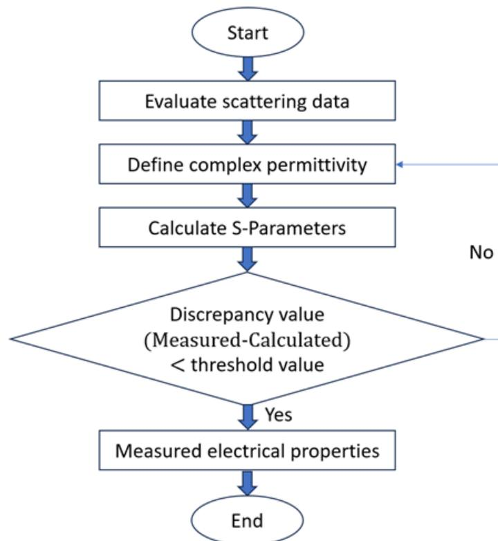
Fig. 3. Material characterization technique
