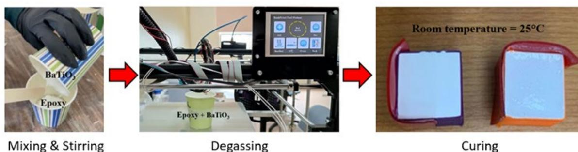
**Fig. 1.** Preparation of composite material
