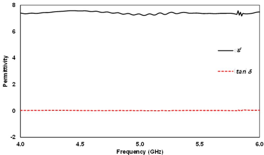
Fig. 5. The permittivity of composite material
