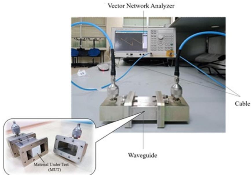
Fig. 2. Measurement setup
