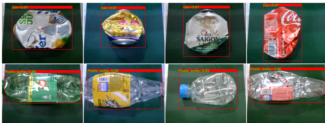
Fig. 7. Classification results: bounding boxes with the center of the object, label classes, and probability
