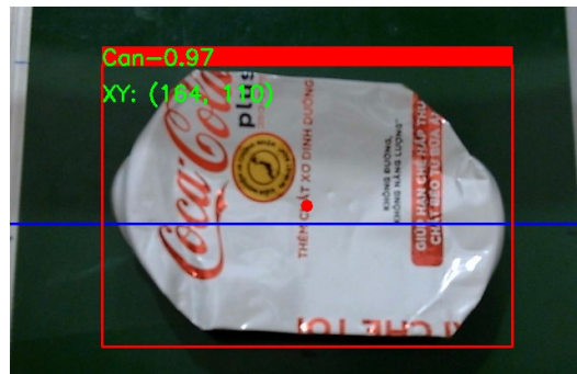
Fig. 4. Determining the coordinates of the picking point
