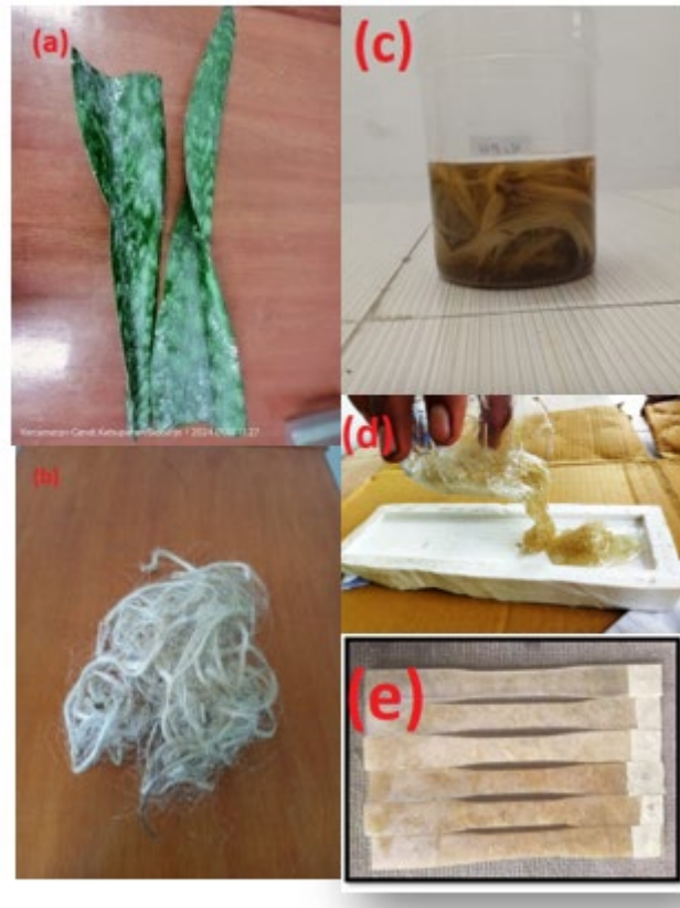
Fig. 4. (a) Fresh sansevieria leaf; (b) Extracted Fibre of Sansevieria (c) NaOH alkalization processes; (d) Hand lay up Composite moulding (e) Composite of sansevieria fibre
