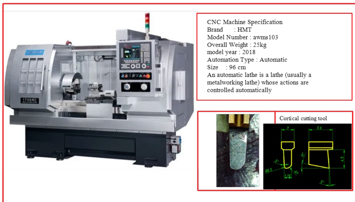
Fig. 1. CNC lathe and cortical cutting tool used in this experiment
