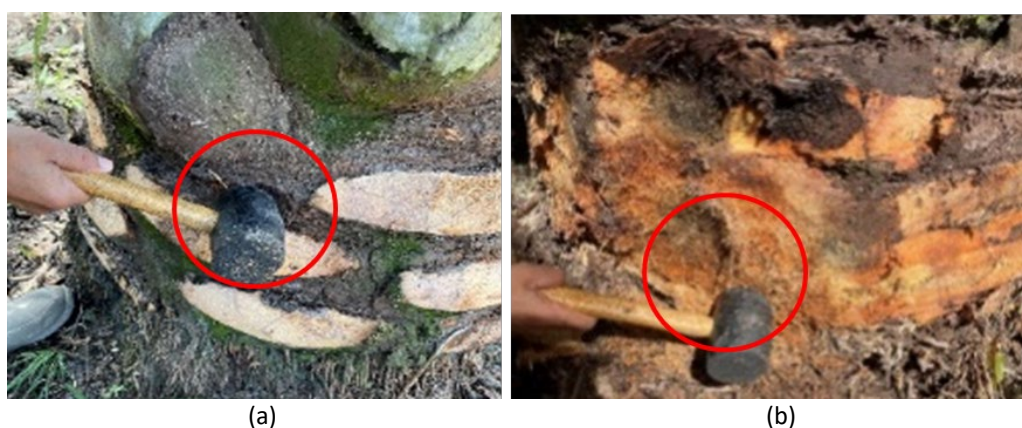
Fig. 2. The experimental setup when collecting the knocking sound data from (a) healthy area (b) the infected area
