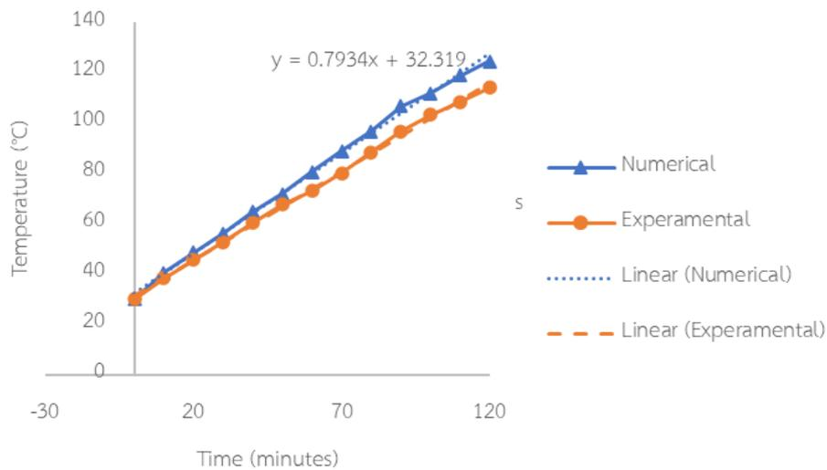
**Fig. 8.** Variation of rubber boots mold surface temperature for inner mold
