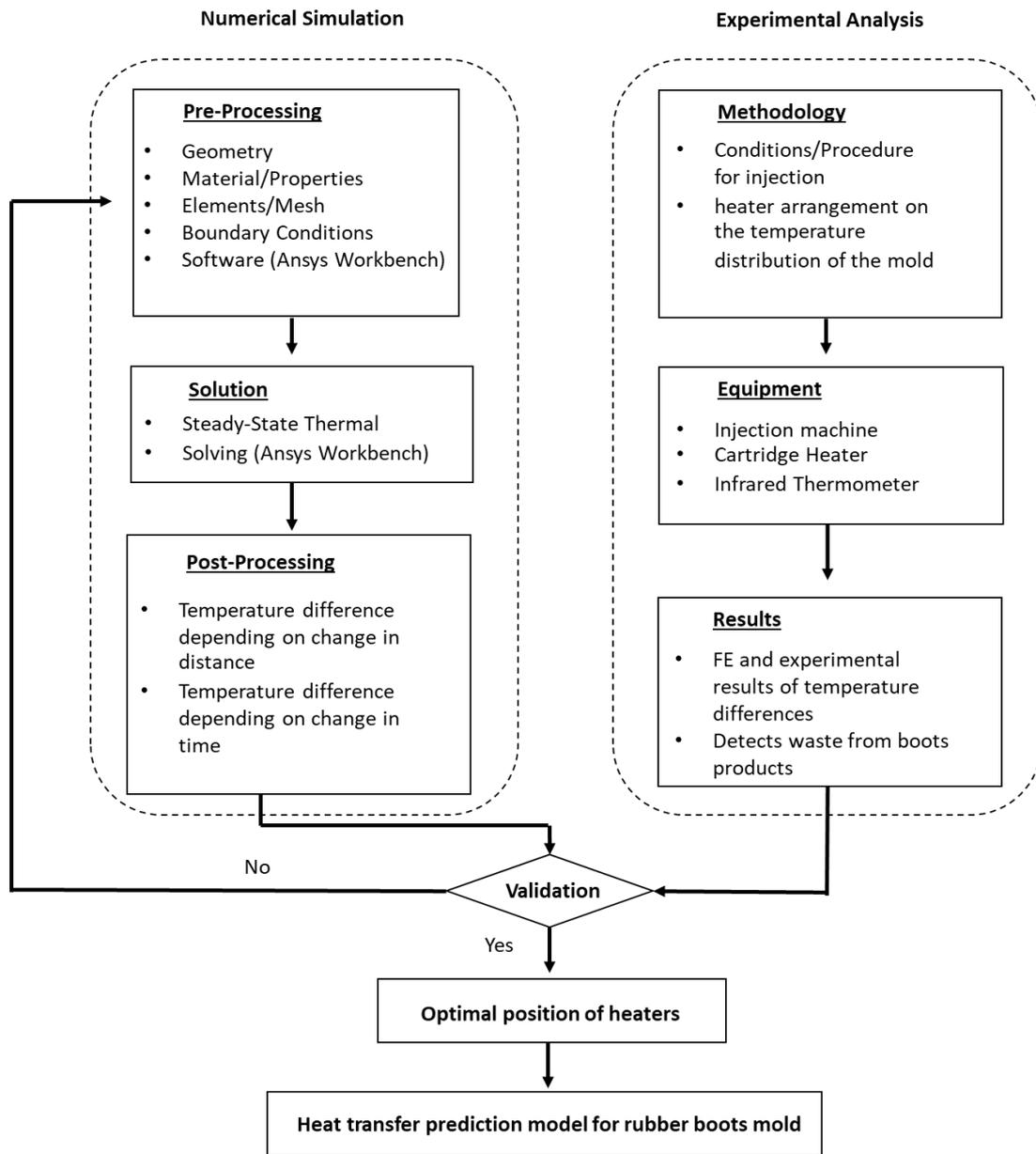
**Fig. 1.** Overall procedure of heat transfer in mold prediction model development for natural rubber boot product
