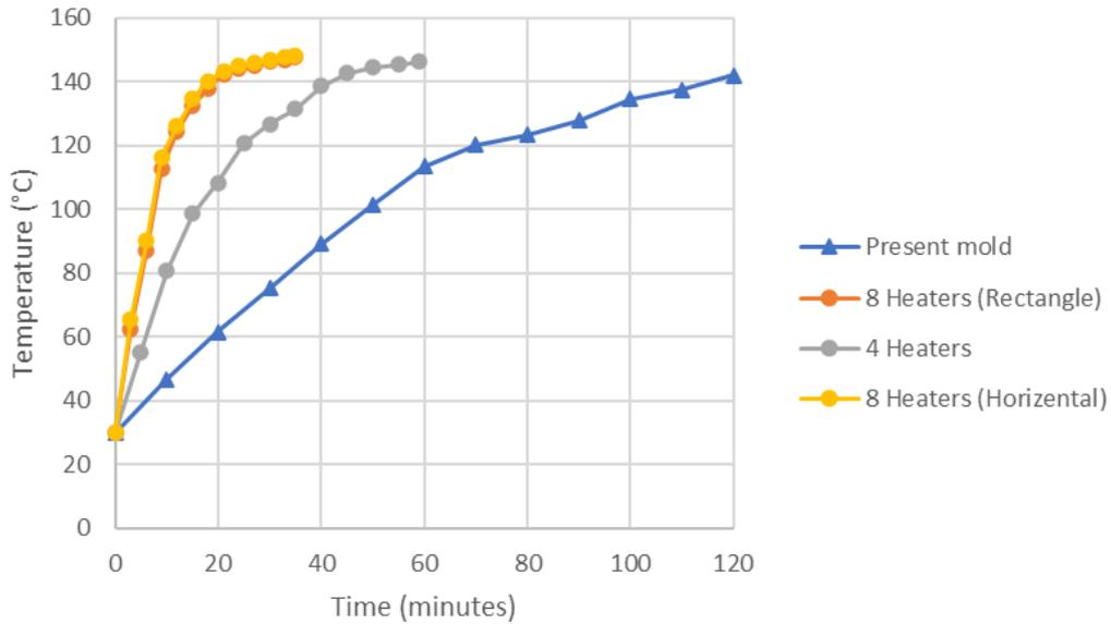
**Fig. 6.** A graph showing the relationship between temperature and time of the outer mold
