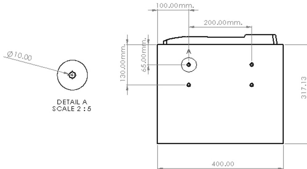
**Fig. 7.** Dimensions of Drill 8 holes in the left-right molds (Improve)
