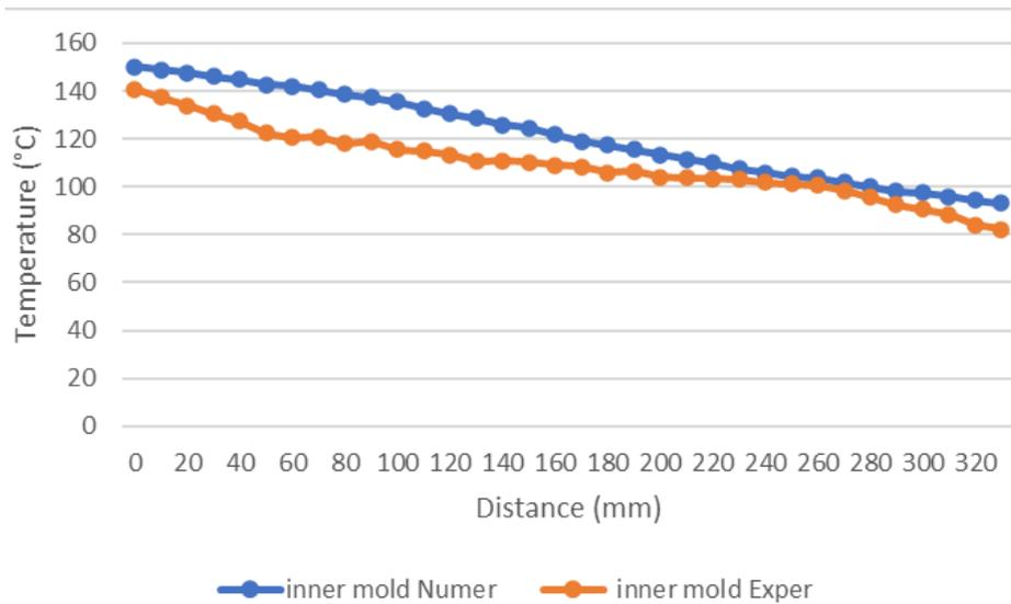
Fig. 10. Variation of rubber boots mold surface temperature for inner mold
