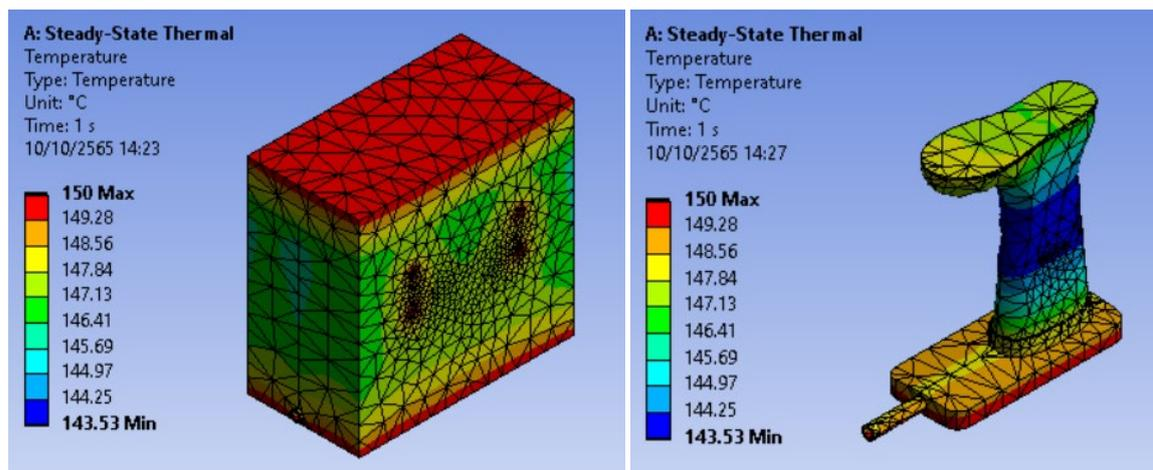
**Fig. 3.** FE model for rubber boots mold
