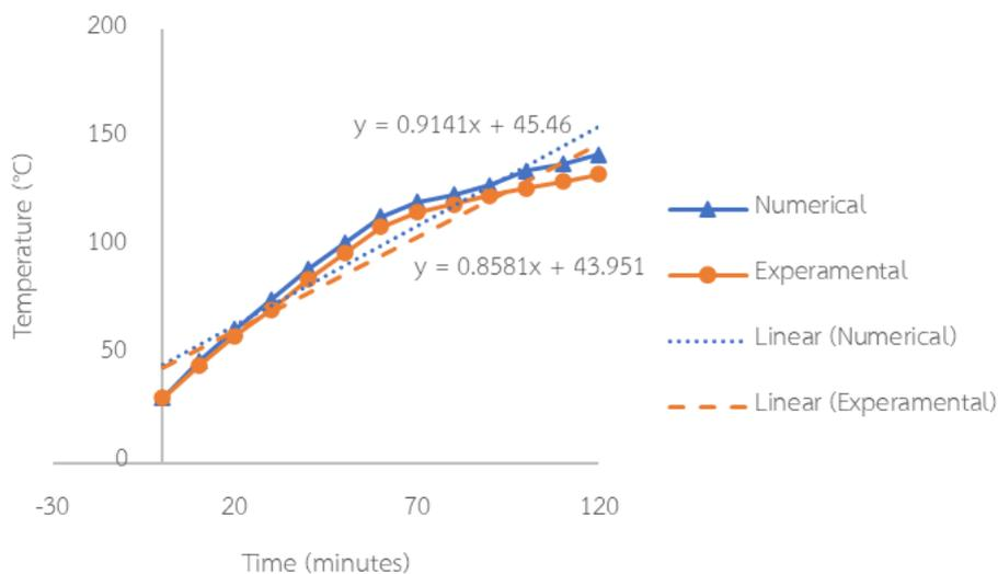
**Fig. 9.** Variation of rubber boots mold surface temperature for outer mold
