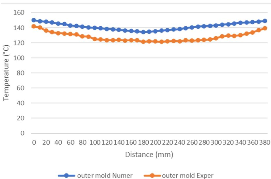
Fig. 11. Variation of rubber boots mold surface temperature for outer mold
