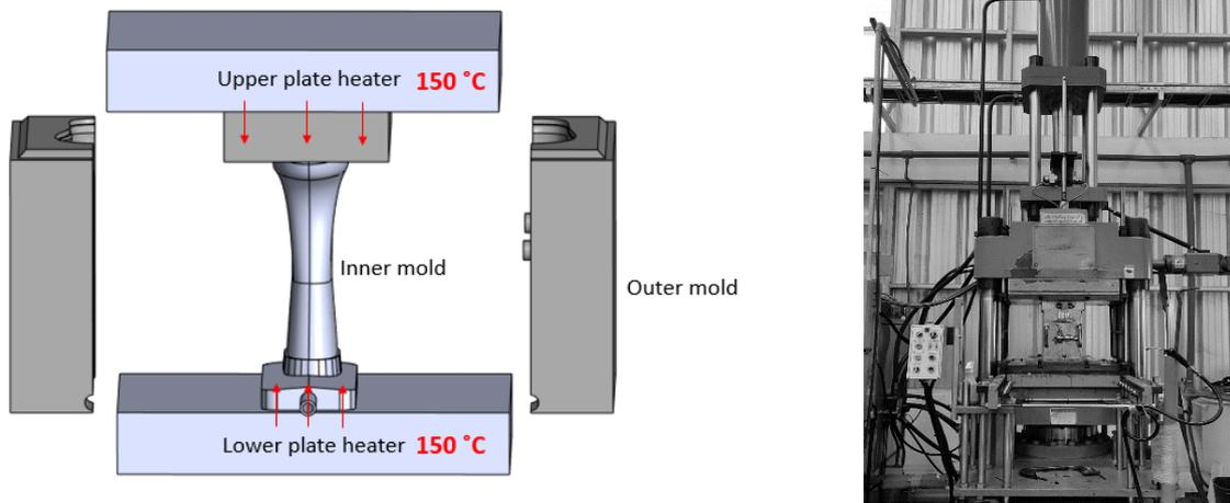
Fig. 4. Equipment and boots mold for rubber injection
