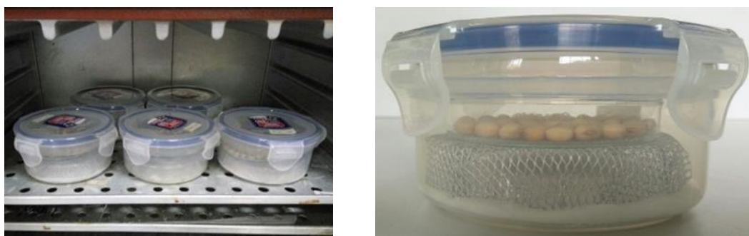
Fig. 1. Soybean seeds sorption isotherm experiment using several saturated salts
