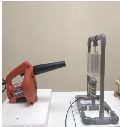
Fig. 10. The position of the blower to the Savonius turbine
