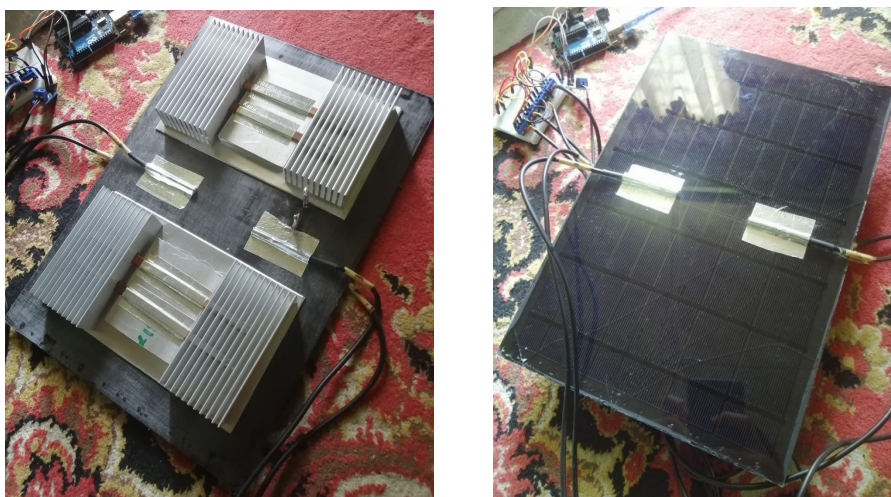
Fig. 2. Fabrication of passive cooling system (left) and placing the temperature sensor (right)
