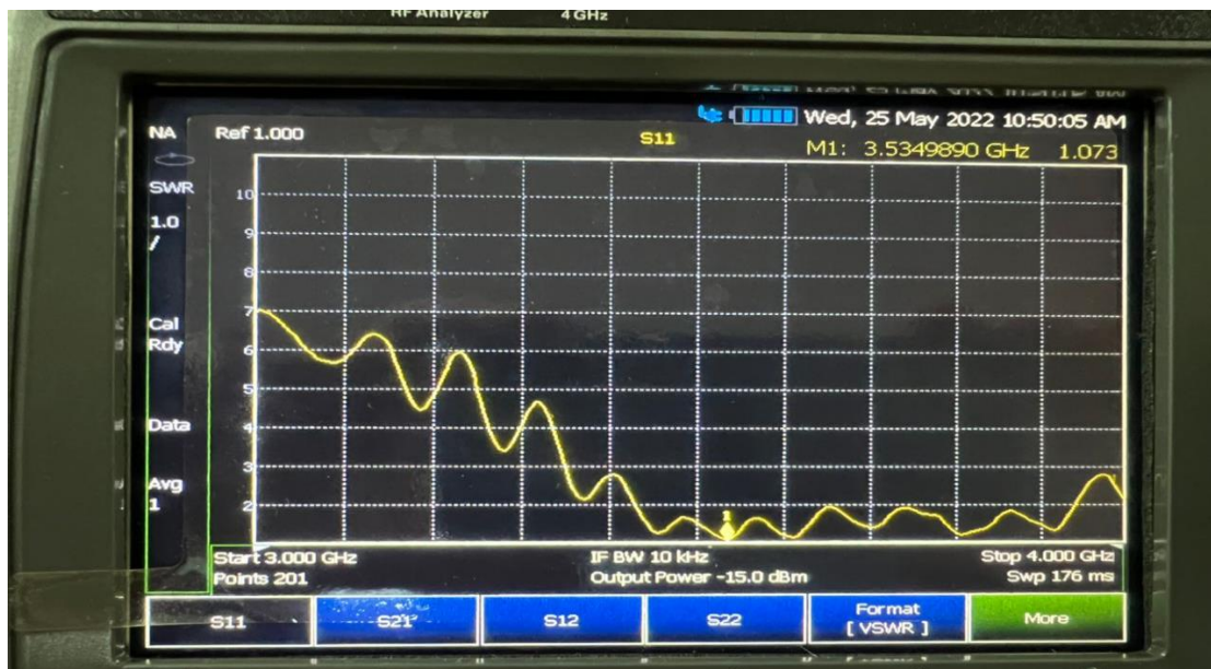
Fig. 14. Measurement of Voltage Standing Wave Ratio (VSWR) of return loss
