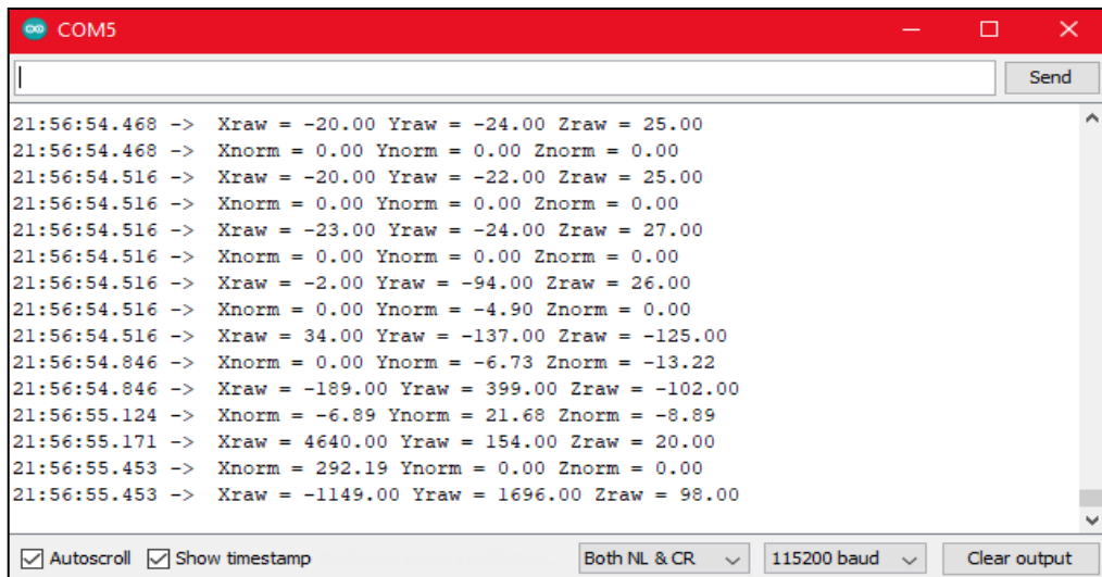
Fig. 5. Serial Monitor display shows the tremor's outcome based on the coordinates of the X, Y, and Z axes to show the earth's instability
