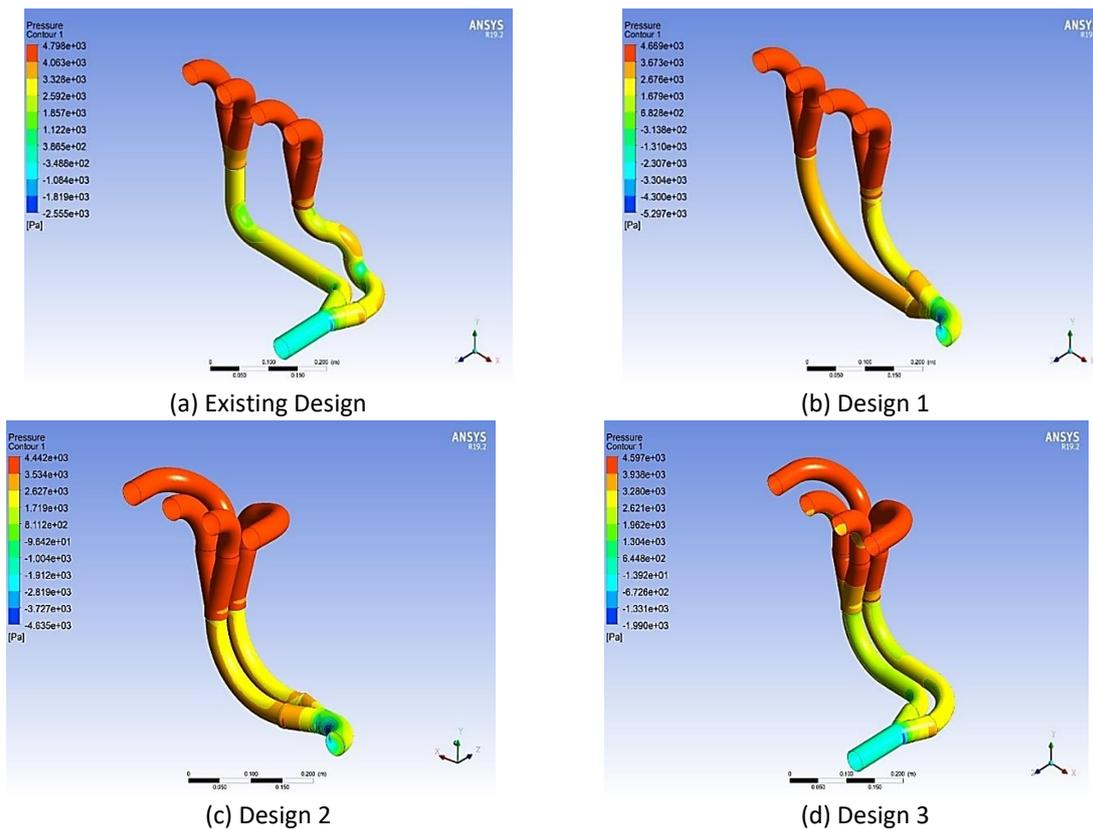
**Fig. 11.** Pressure Contour of each design of the exhaust manifold
