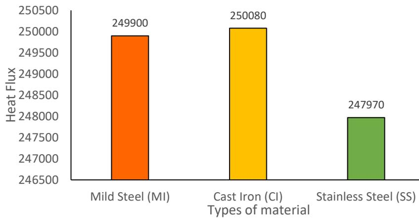
Fig. 8. Maximum heat flux at time period of 30 seconds
