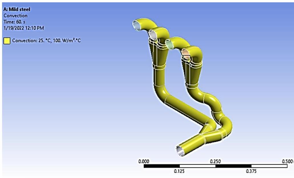
Fig. 3. Convection was applied on the outer surface of the geometry
