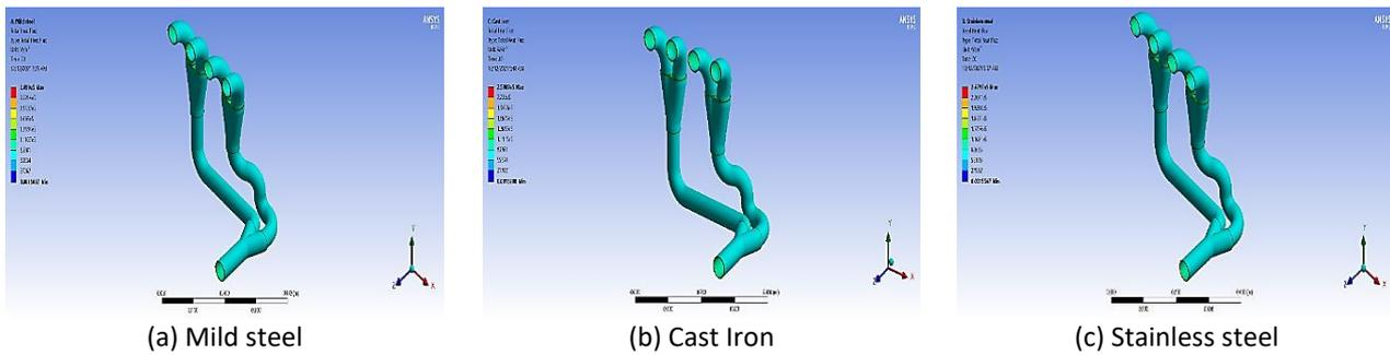
Fig. 7. Temperature distribution of three materials on the exhaust manifold
