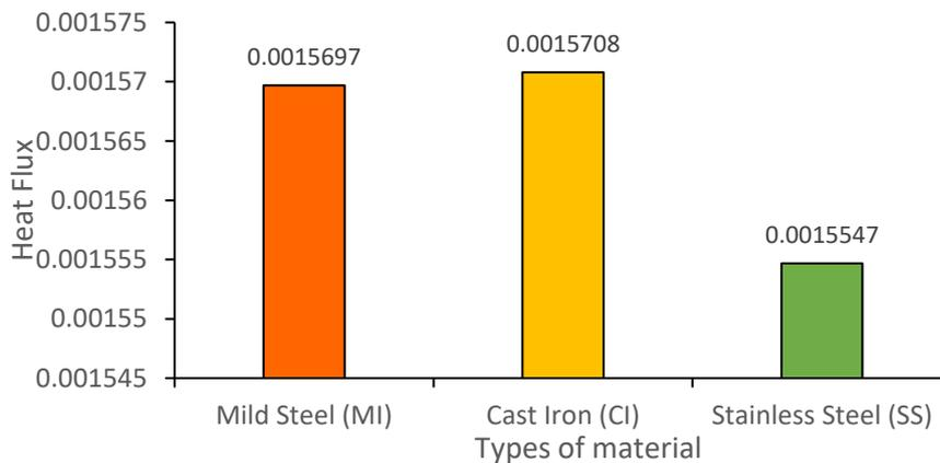
Fig. 9. Minimum heat flux at time period of 30 seconds
