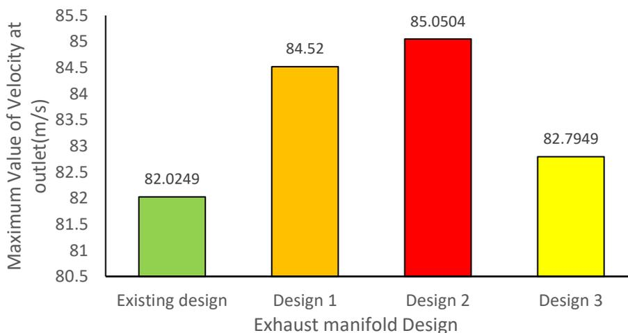
**Fig. 12.** Graph of comparison in velocity at outlet
