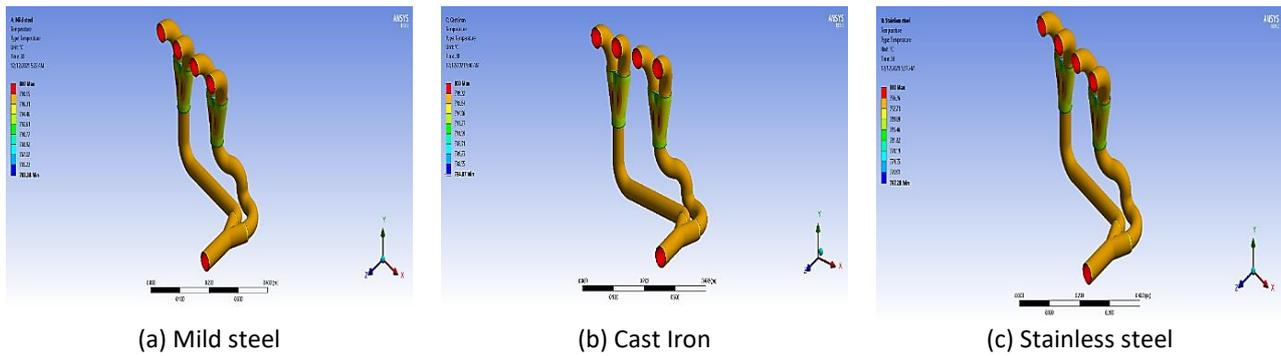
**Fig. 5.** Temperature distribution of three materials on the exhaust manifold
