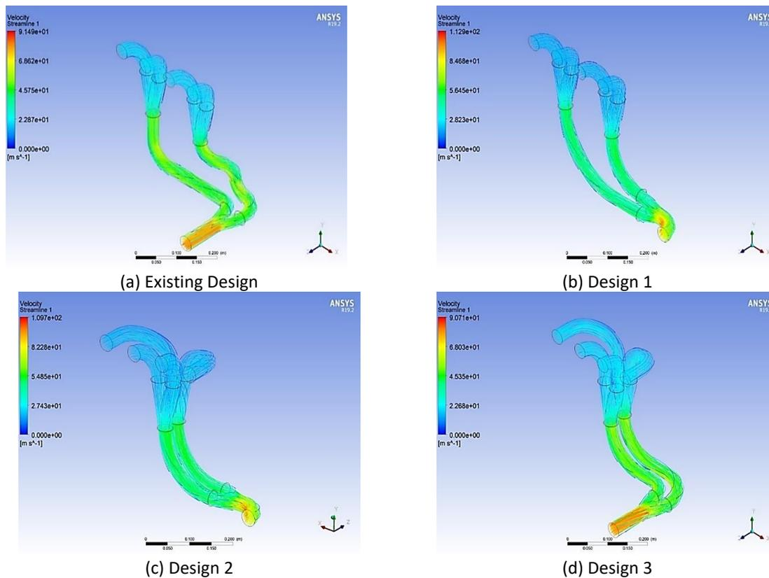
**Fig. 10.** Velocity streamlines of each design of the exhaust manifold
