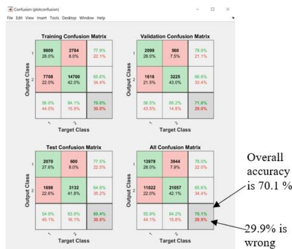
Fig. 7. Plot of Confusion Matrix for training, validation, test and overall confusion for Data 1 of RC A at ANN in MATLAB.
