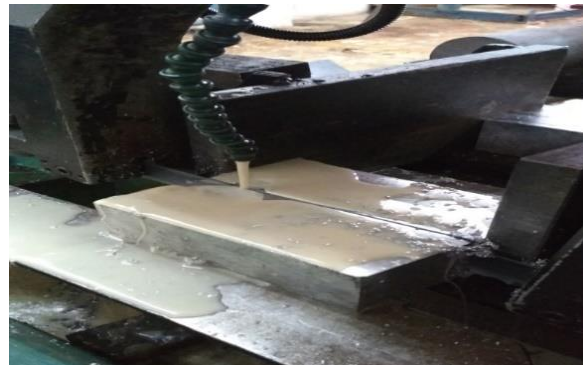
Fig. 3. Cutting material with bend saw machine
