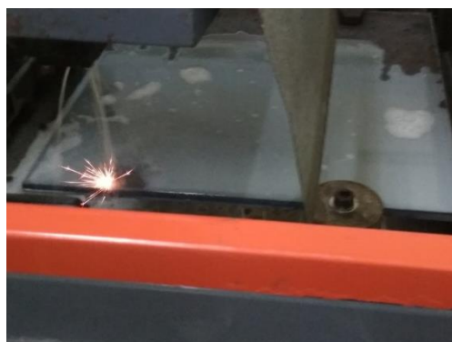
Fig. 7. Cutting outer shape of base plate
