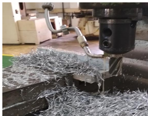
Fig. 4. Removing material to form L shape
