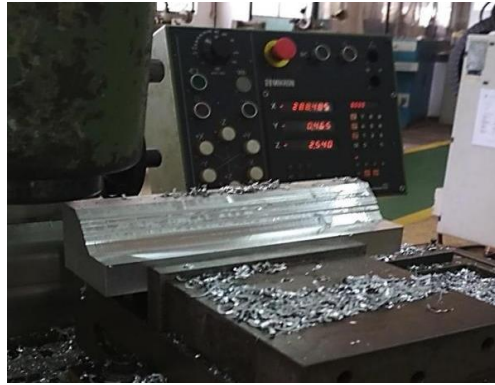
Fig. 5. Cutting slot at top and side surface
