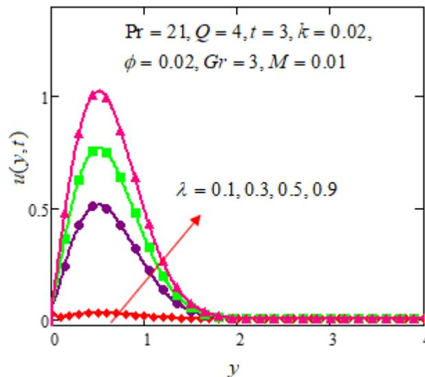
Fig. 5. Velocity profile for different values of Maxwell parameter  $\lambda$
