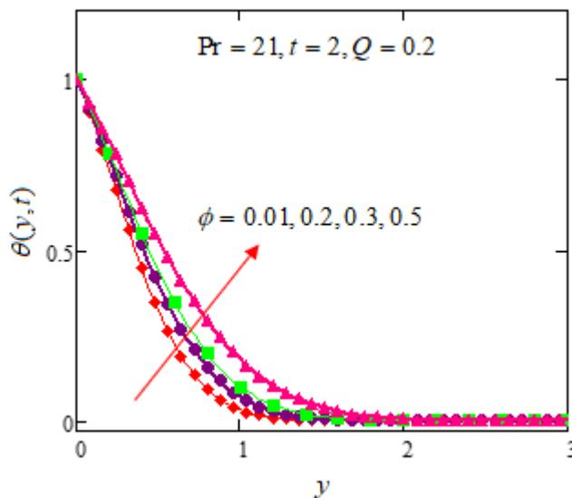
Fig. 3. Temperature profile for various values of volume fraction  $\phi$
