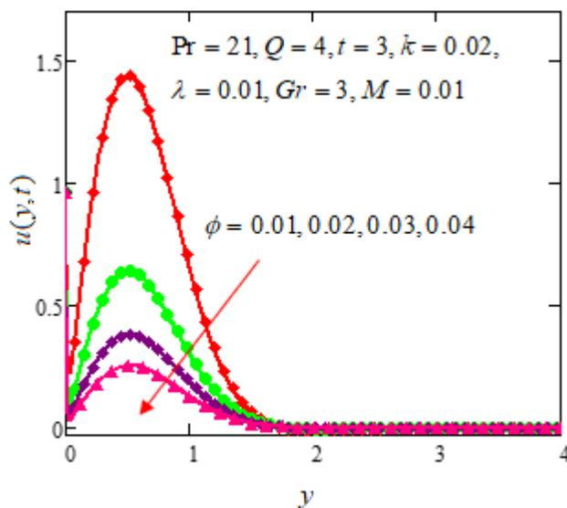
Fig. 4. Velocity profile for different values of volume fraction  $\phi$
