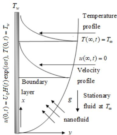
Fig. 1. Geometry of the flow over a vertical plate
