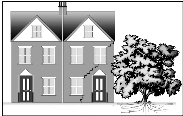
Fig. 14. Root of trees can lead to cracks on buildings
