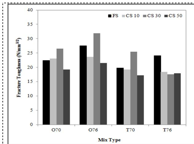
Fig. 10. Effects of clogging on fracture toughness
