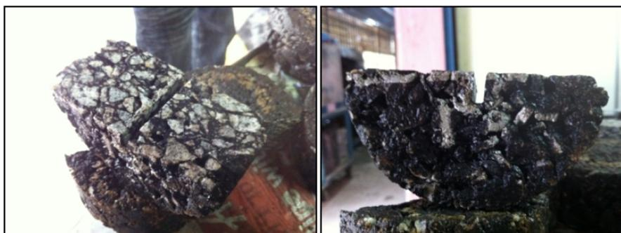
**Fig. 3.** Specimen prepared for SCB test
