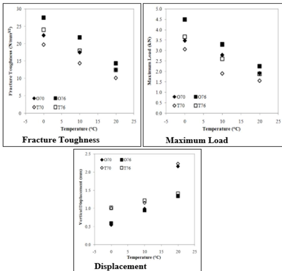
Fig. 6. Effects of temperature on fracture toughness, Maximum load and displacement
