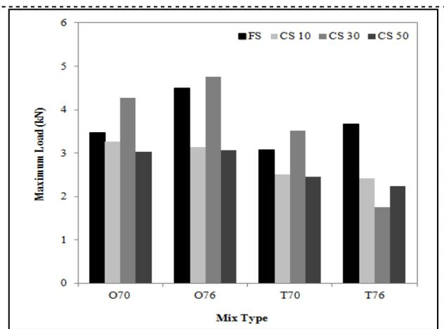
Fig. 11. Effects of clogging on maximum load
