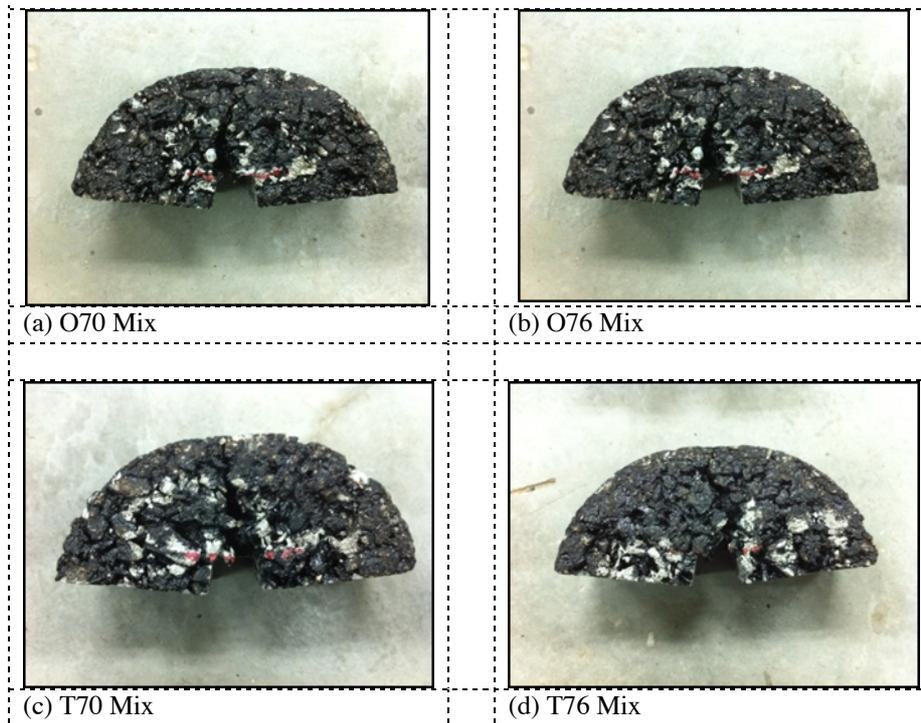
Fig. 4. Fresh specimens tested at 0°C
