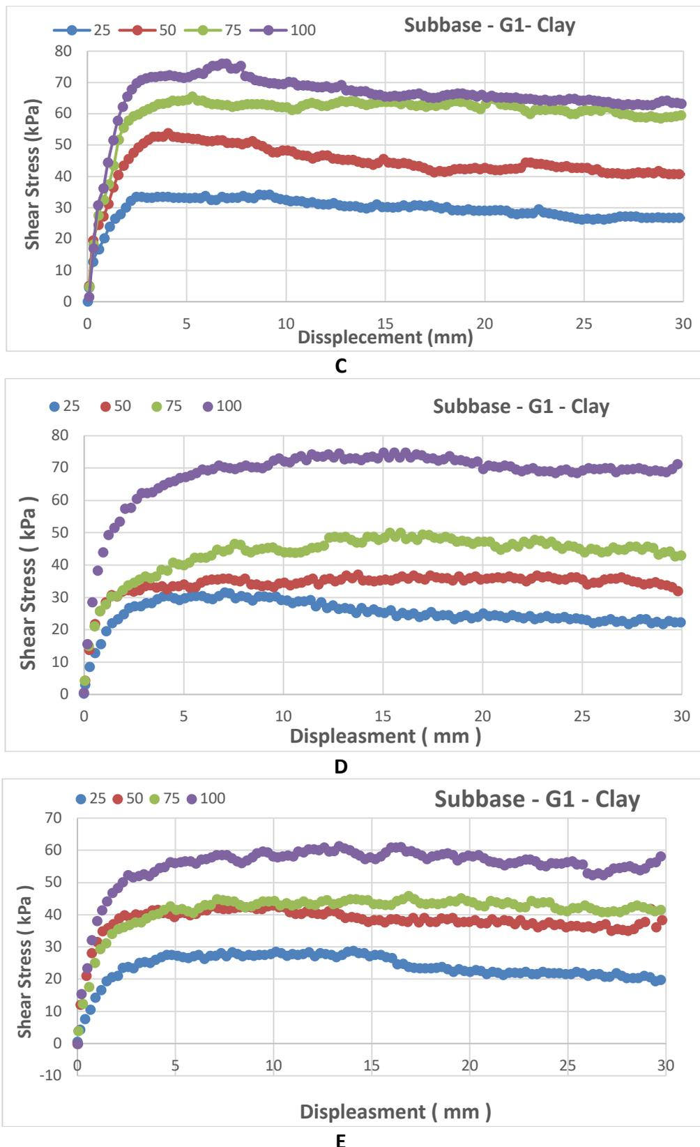
**Fig. 7.** Shear stress with displacement for 100% degree of compaction and water content (6,8,10,12 and 14% respectively) with G1
