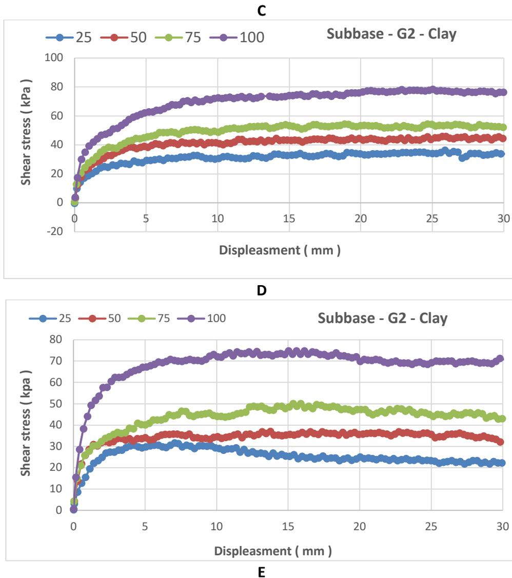
**Fig. 8.** Shear stress with displacement for 100% degree of compaction and water content (6,8,10,12 and 14% respectively) with G2
