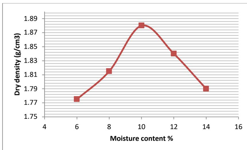
**Fig. 1.** Compaction curve of the clay subgrade soil
