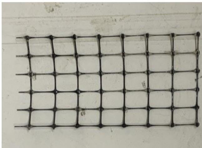
**Fig. 4.** Geogrid reinforcement (SS2)
