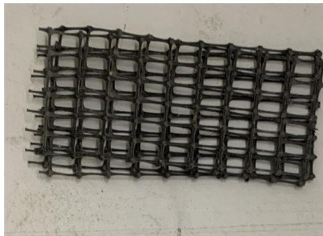
Fig. 3. Geogrid reinforcement (BX1100)
