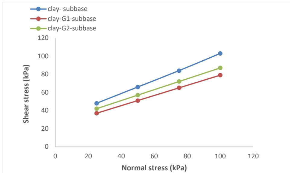
**Fig. 11.** Peak shear envelope of the soil at optimum state
