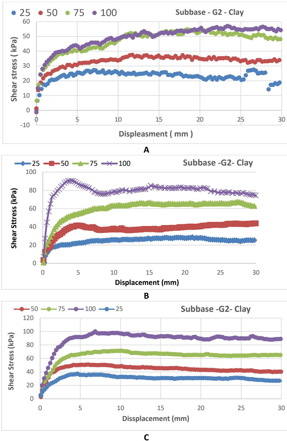
**Fig. 10.** shear stress with displacement for 10% water content and degree of compaction (90%, 95% and 98% respectively) with G2
