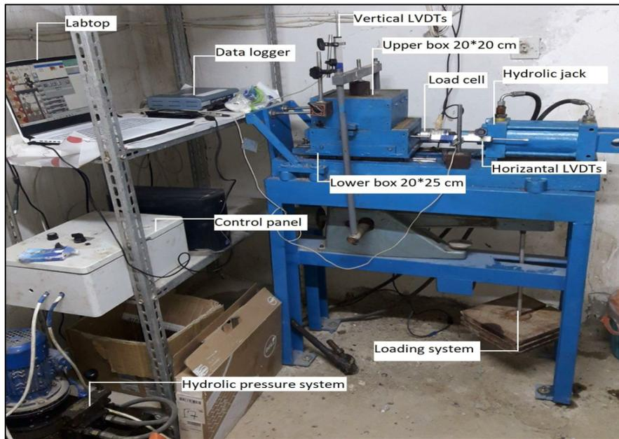
Fig. 5. Large-scale direct shear apparatus
