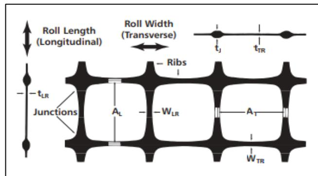
Fig. 2. Details of geogrid reinforcement SS2 (Tensar international company's)
