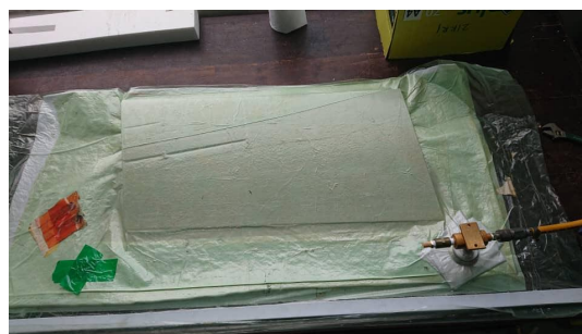
Fig. 5. Vacuum bagging of the wing
