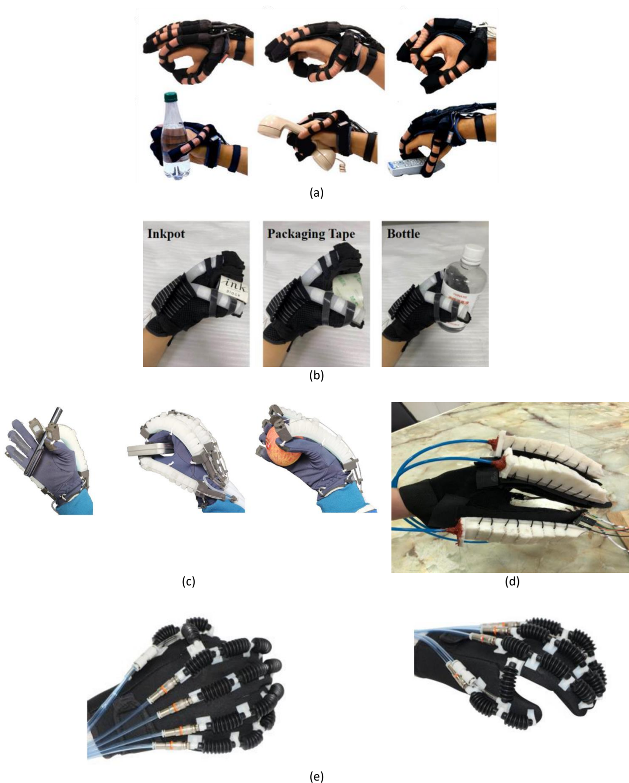
Fig. 2. Soft gloves for both rehabilitation and assistance (a) hydraulic soft robotic glove with soft fibre-reinforcement actuators [14] (b) pneumatic customized soft glove with bioinspired segmented hybrid bending actuators (SHBAs) [21] (c) bidirectional soft glove with a hybrid actuator that combines a silicone flexion actuator with an extension actuator made from shape memory alloy (SMA) springs [23] (d) KNTU-RoboGlove: The soft glove integrates with variable stiffness layer actuators, drawing inspiration from pangolins [24] (e) A novel soft robotic glove with positive-negative pneumatic actuator mode of bel
