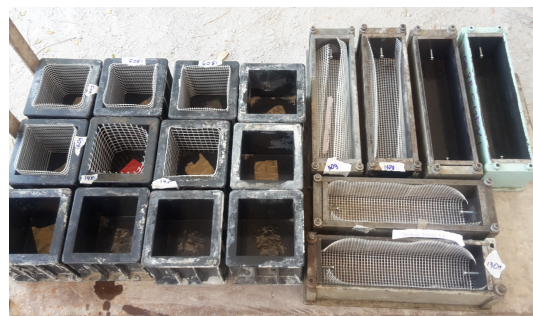
Fig. 1. Alkali-resistant woven fibre meshes were positioned in the steel mould
