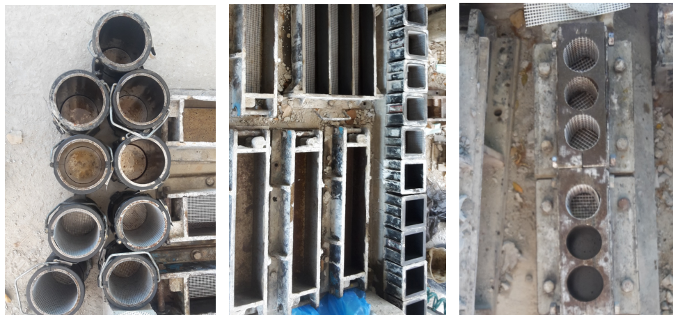
Fig. 1. Fibreglass fabrics were placed accordingly in the steel moulds
