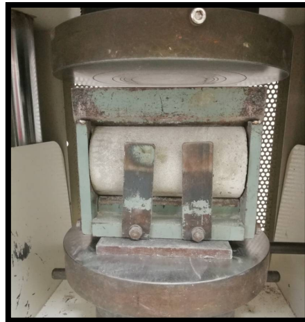
Fig. 4. Splitting tensile strength test setup measurement based on ASTM C496
