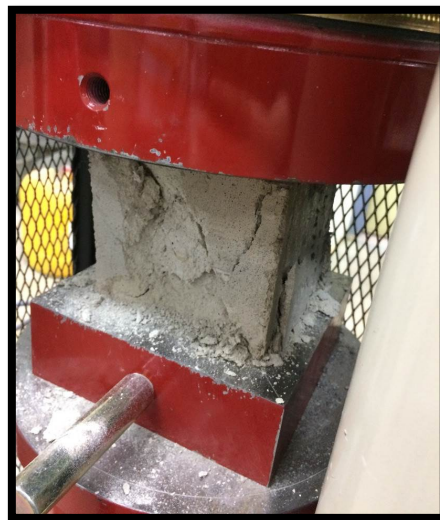
Fig. 2. Compression test setup in accordance with BS12390
