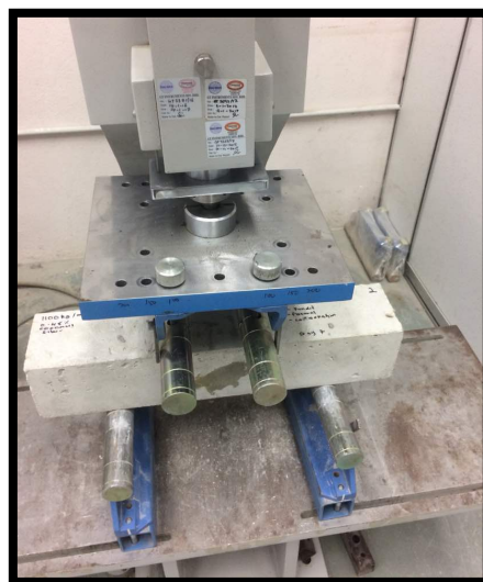
Fig. 3. Bending test setup corresponding to BS1521
