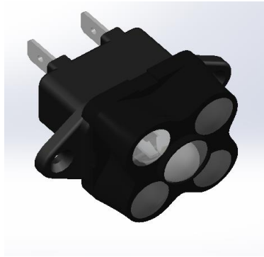
Fig. 5. Proposed design for portable wireless parking sensor device developed in SolidWorks.
