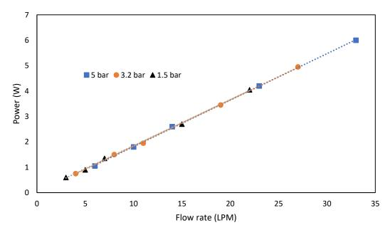
Fig. 14. Flow rate vs Power for a different working pressure
