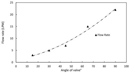
Fig. 10. Low-rate vs Angle of valve for 1.5 bar working pressure
