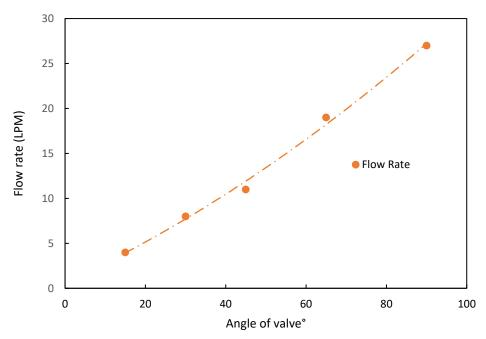
Fig. 6. Flow rate vs Angle of valve for 3.2 bar working pressure
