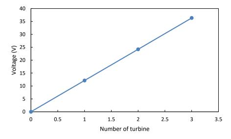
Fig. 21. Number of turbines vs voltage produced
