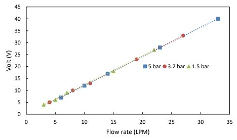
Fig. 16. Flow rate vs Volt for a different working pressure
