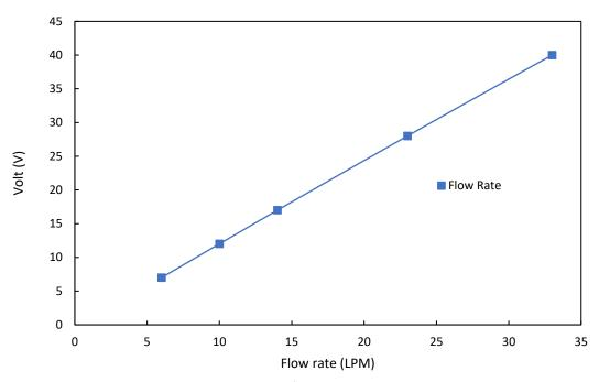
Fig. 3. Flow rate vs Volt for 5 bar working pressure
