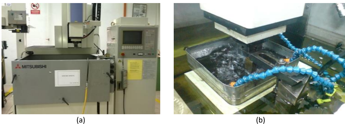
Fig. 4. (a) MITSUBISHI EX22 die-sinking EDM, (b) Experimental setup for Die Sinking EDM
