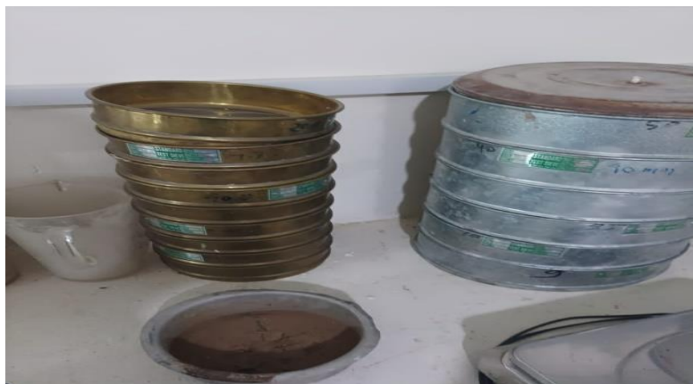
Fig. 7. Sieve analysis in the SIMAD lab
