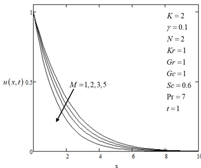
**Fig. 3.** Velocity profiles for various values of  $M$
