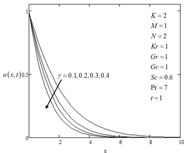
**Fig. 4.** Velocity profiles for various values of  $\gamma$
