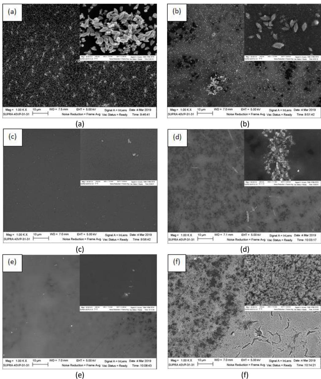
**Fig. 2.** FESEM image of ZnO nanostructure doped with Niobium with different mass percentage (a) 5wt% (b) 10wt% (c) 15wt% (d) 20wt% (e) 25wt% and (e) undoped ZnO
