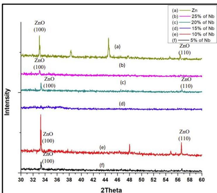
**Fig. 3.** X-ray diffraction pattern of the ZnO particle on thin film with different ratio mass percentage of dopant at range  $2\theta$  between  $30^\circ - 60^\circ$
