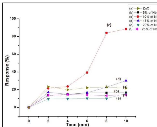
**Fig. 4.** The responses of the ZnO nanoparticles doped Nb exposed to the Argon gas in 10 minutes at room temperature
