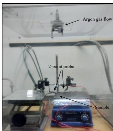
**Fig. 1.** Experimental set-up for gas testing
