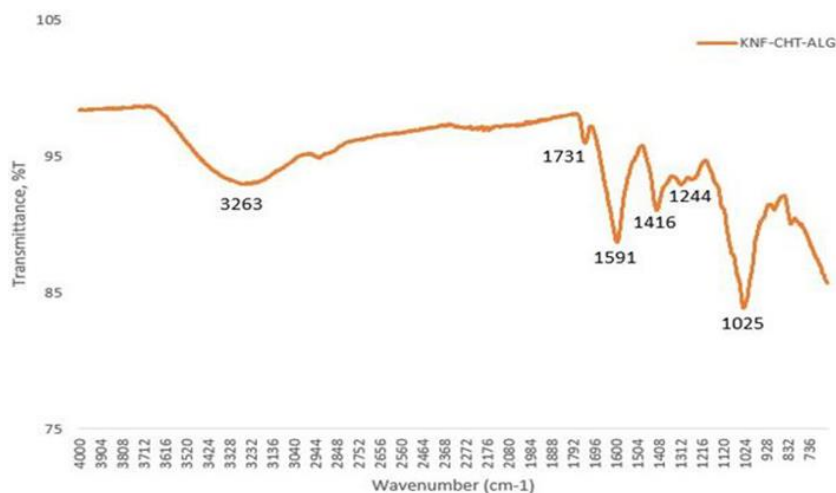
Fig. 2. FTIR spectra of the KNF-CHT-ALG beads within the 700–4000 cm -1 scanning range
