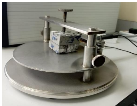
Fig. 2. Hot Disk TPS 2500S for thermal properties measurement
