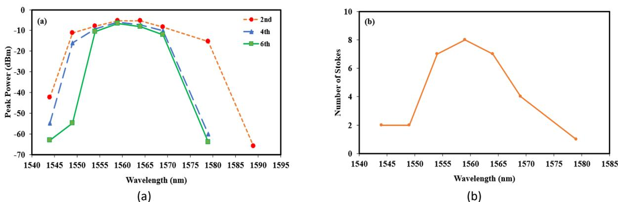
**Fig. 5.** (a) Tuning Characteristics of the DF-MWBEFL (b) number of generated Brillouin Stokes lines against BP wavelength
