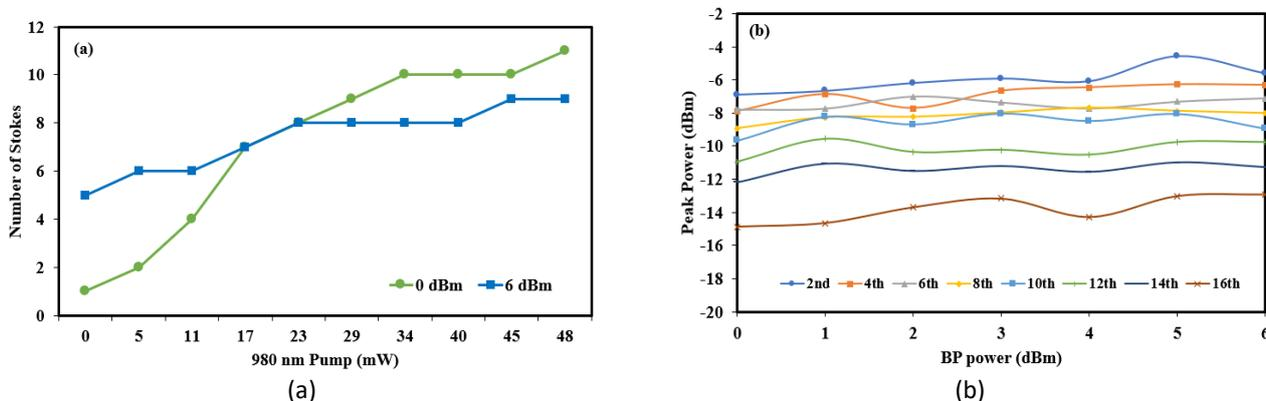
**Fig. 4.** (a) Number of generated double-frequency spacing Brillouin Stoke at various 980 nm pump power and BP power (b) Brillouin Stokes power of the DF- MWBEFL at different BP power
