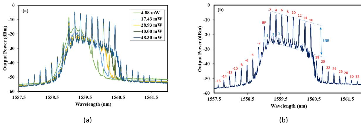
**Fig. 2.** (a) Optical spectra of the DF- MWBEFL at various 980nm pump power (b) DF-MWBEFL spectrum with maximum number of generated Brillouin Stokes lines
