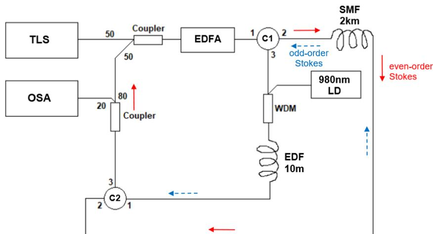
Fig. 1. Schematic of the double-frequency spacing BEFL
